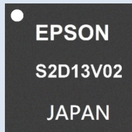
A S2D13V02 (in a P-TFBGA-081-0808-0.80 package)
