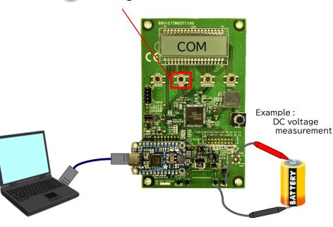
When reading is completed, a "Logs" folder will be created and the measurement data "Output.csv" will be saved in that folder.
