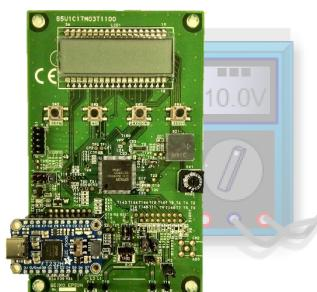
Evaluation board of MCU "S1C17M03" for digital multimeter
