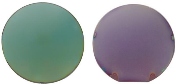
Fig. 1.8 Color Unevenness on Wafer Back Side (Macro Visual)
