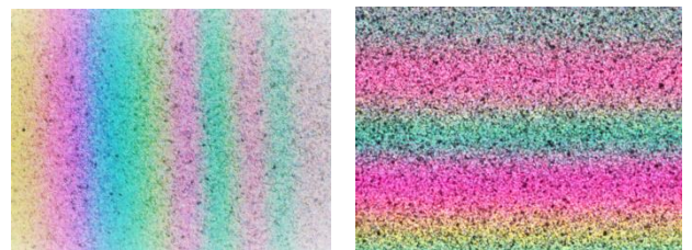
Fig. 1.9 Color Unevenness on Wafer Back Side (Micro Visual)
