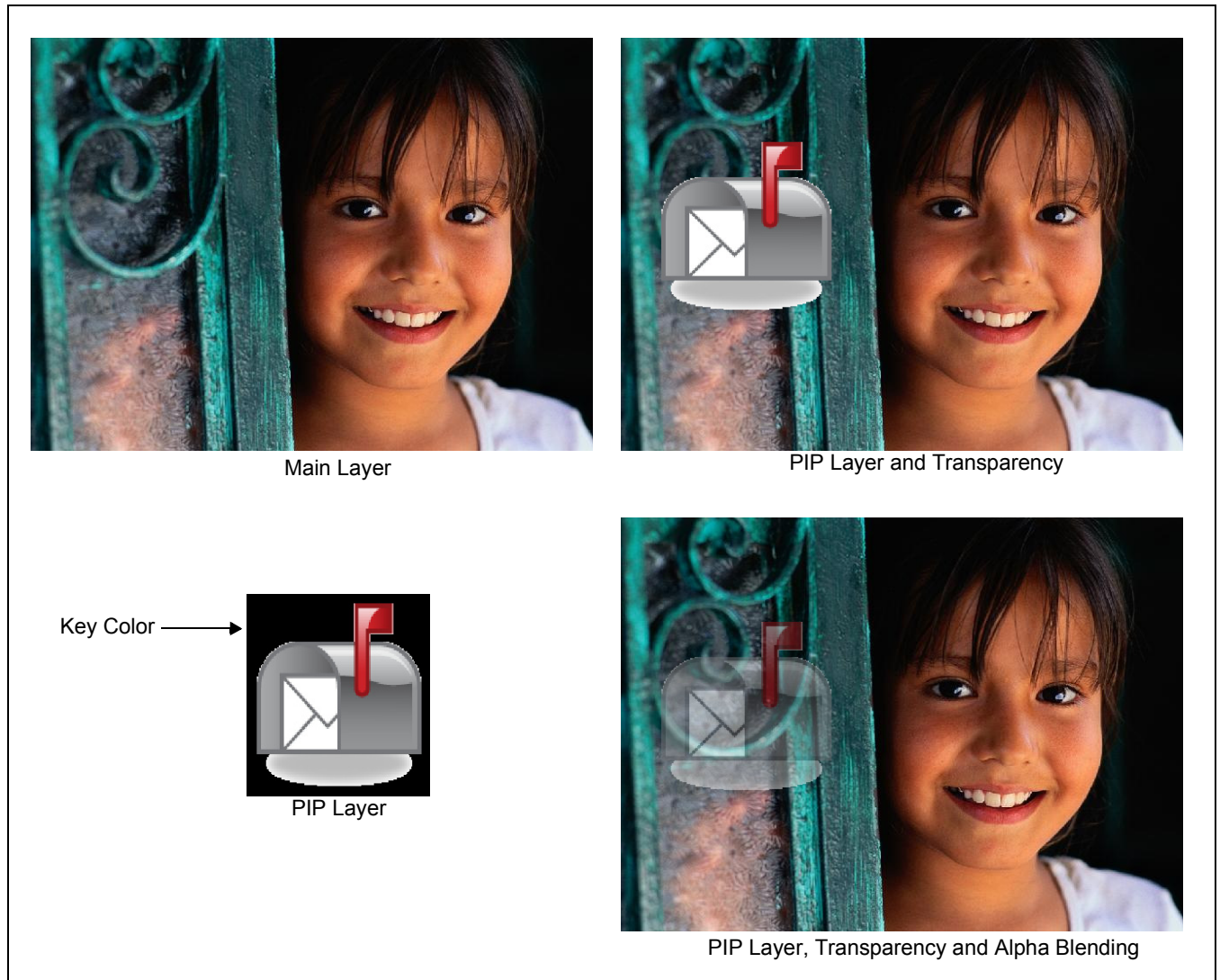
Figure 14-3: PIP Layer Alpha Blending
