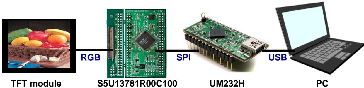
*Figure 4-1 Constitution of Display Demo using a PC*
