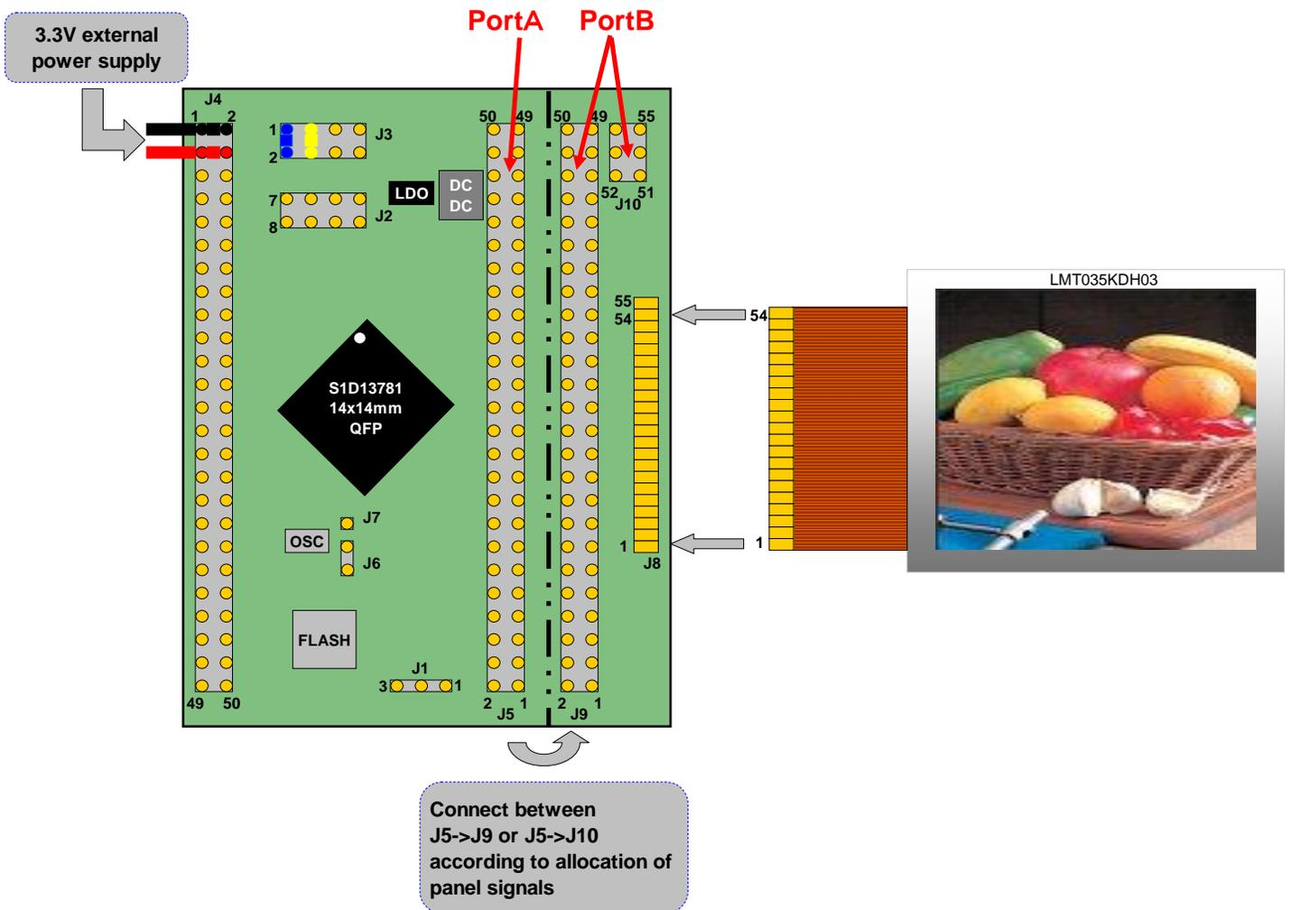
Figure 3-3 LMT035KDH03 Connection Example
