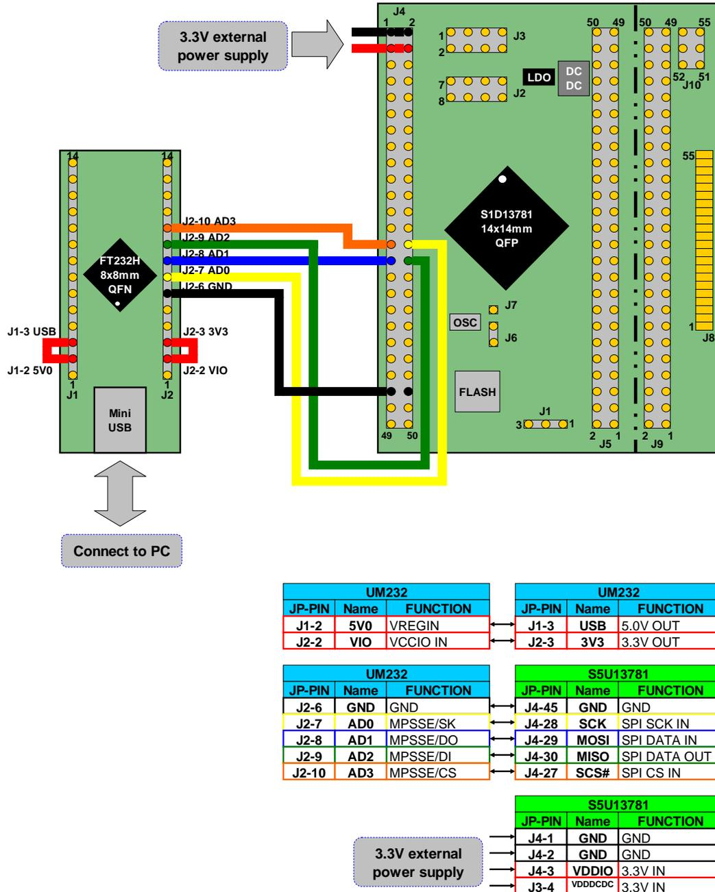
Figure 4-2 Connecting the UM232H to S1D13781 via SPI
