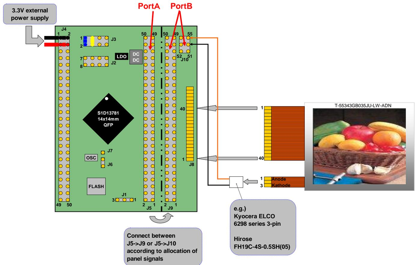
Figure 3-3 T-55343GD035JU-LW-ADN Connection Example
