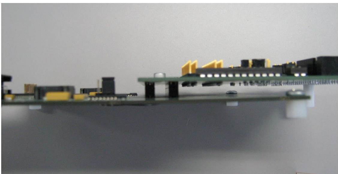
Figure 9.4 Connecting S5U13U00P00C100 Board and S5U13U00P00C100 Board
