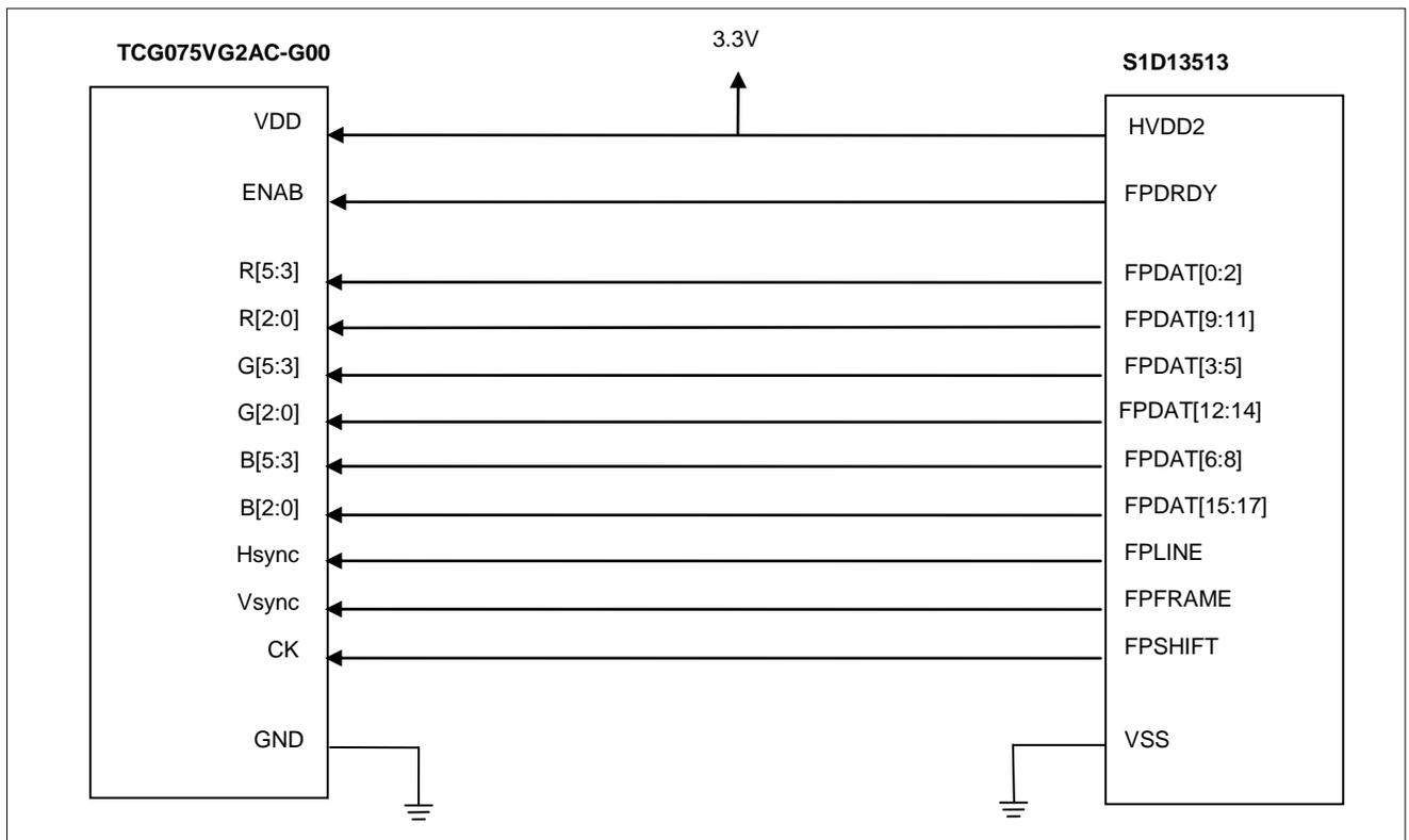
Figure 11-1 Connecting the TCG075VG2AC-G00 to the S1D13513
