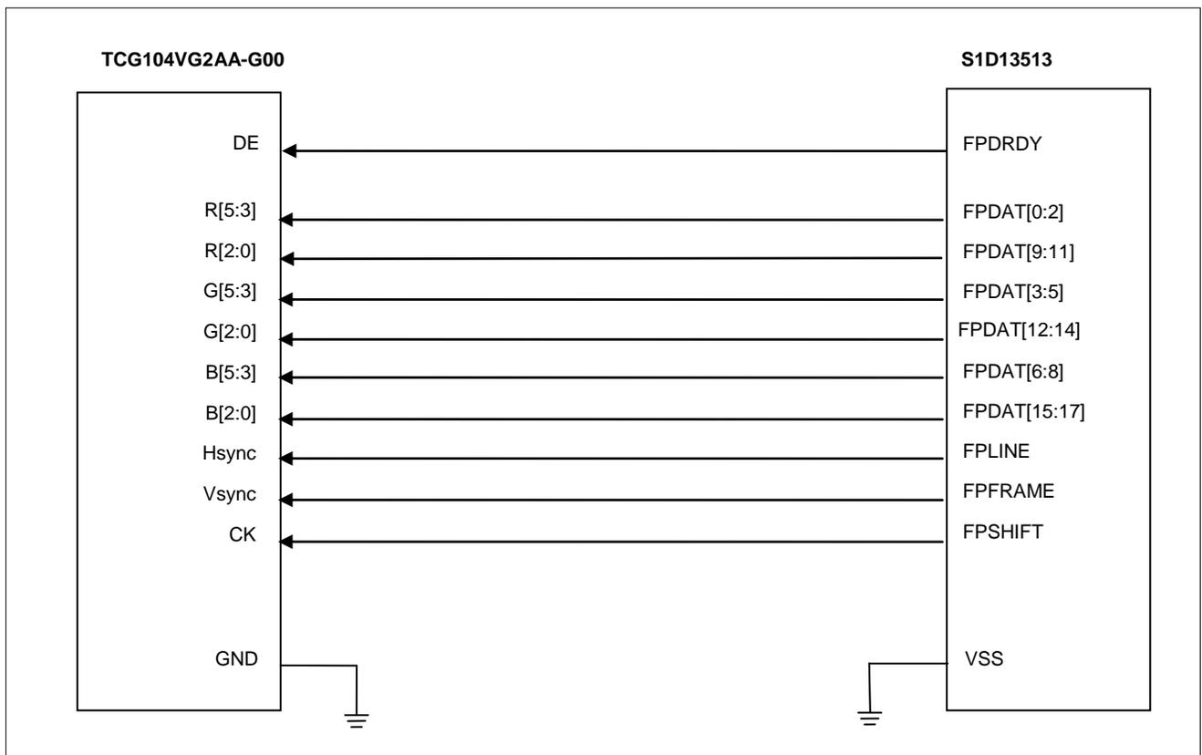
Figure 13-1 Connecting the TCG104VG2AA-G00 to the S1D13513
