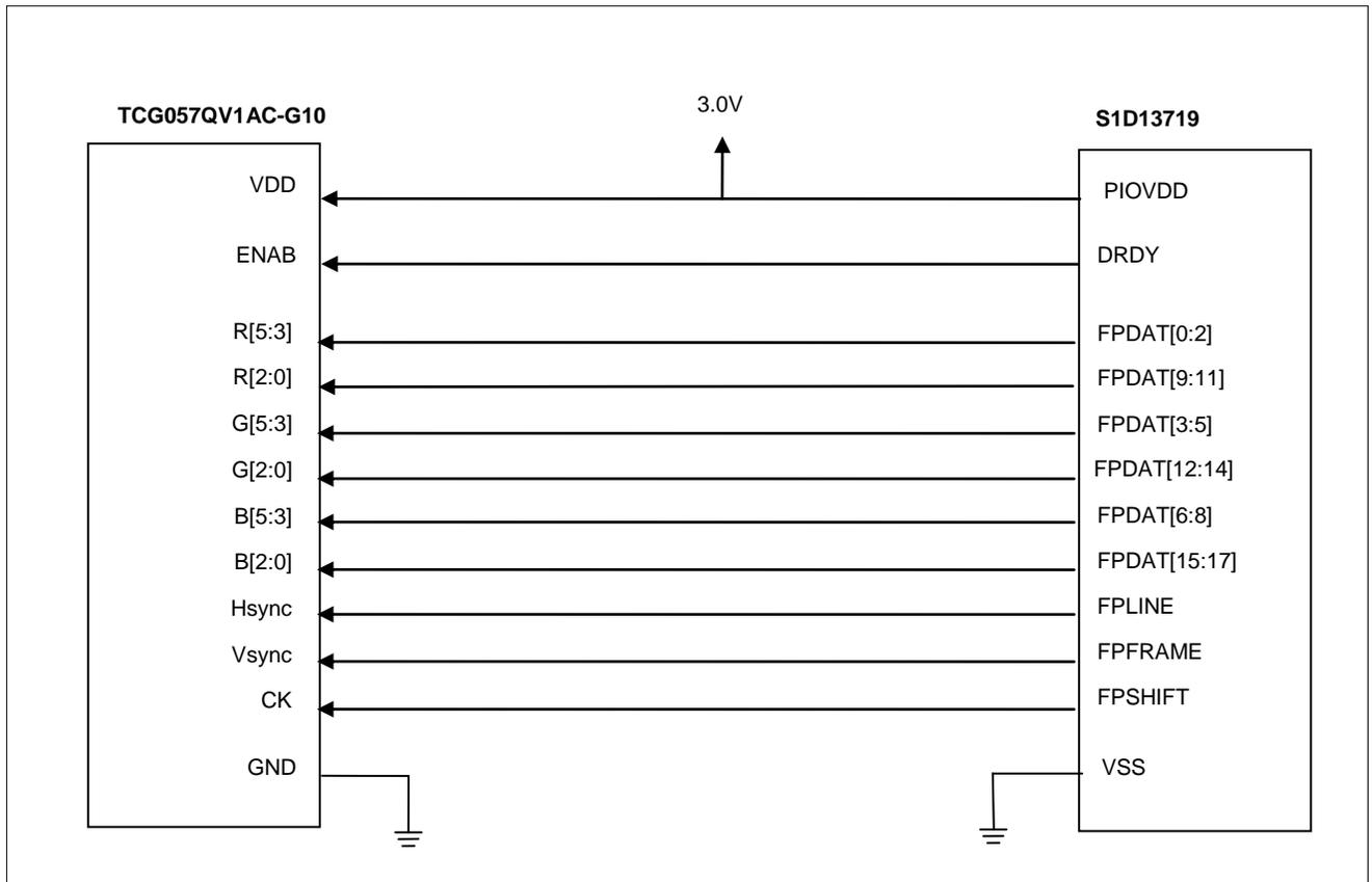
Figure 5-2 Connecting the TCG057QV1AC-G10 to the S1D13719
