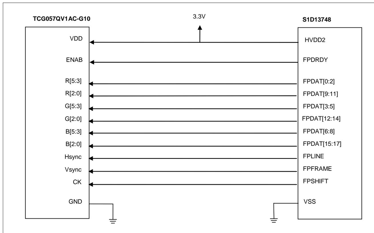
Figure 5-5 Connecting the TCG057QV1AC-G10 to the S1D13748
