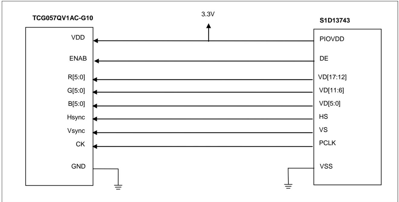
Figure 5-4 Connecting the TCG057QV1AC-G10 to the S1D13743
