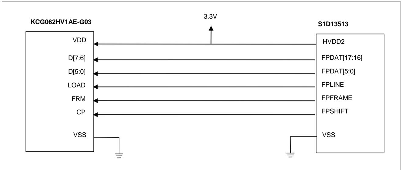
Figure 8-1 Connecting the KCG062HV1AE-G03 to the S1D13513
