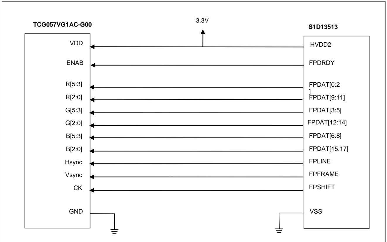
Figure 6-1 Connecting the TCG057VG1AC-G00 to the S1D13513
