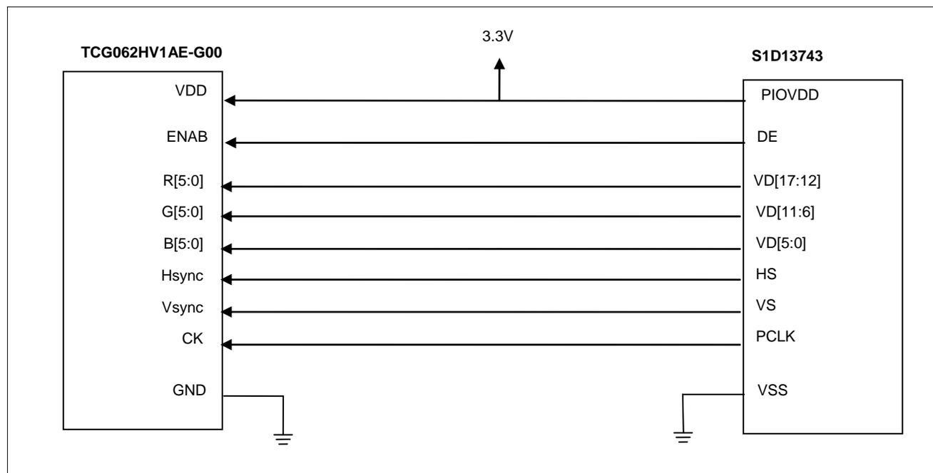
Figure 9-3 Connecting the TCG062HV1AE-G00 to the S1D13743
