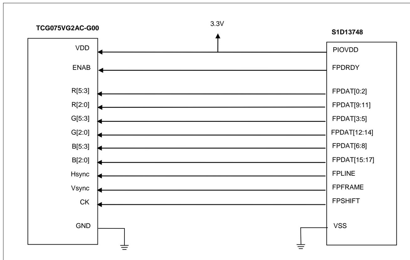
Figure 11-2 Connecting the TCG075VG2AC-G00 to the S1D13748
