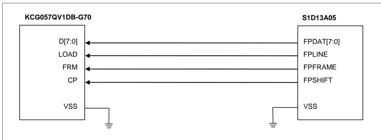
Figure 3-3 Connecting the KCG057QV1DB-G70 to the S1D13A05
