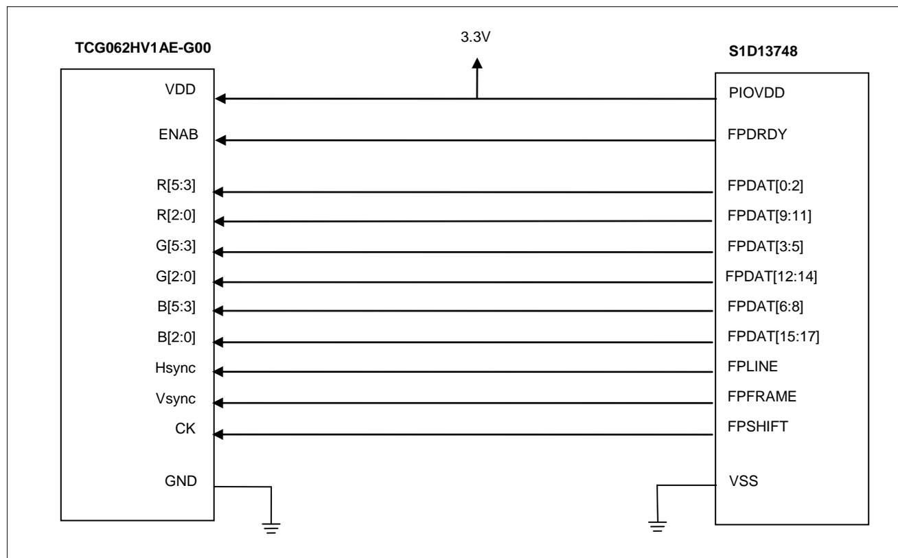
Figure 9-4 Connecting the TCG062HV1AE-G00 to the S1D13748
