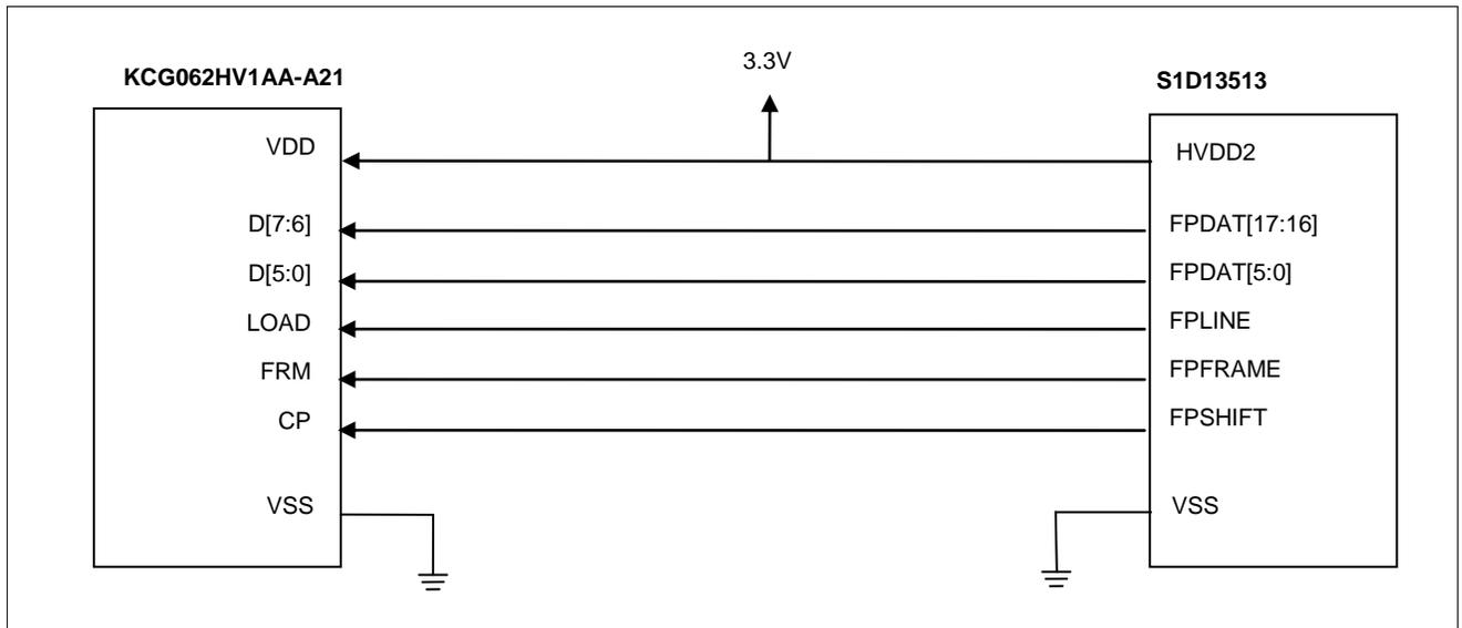
Figure 7-1 Connecting the KCG062HV1AA-A21 to the S1D13513
