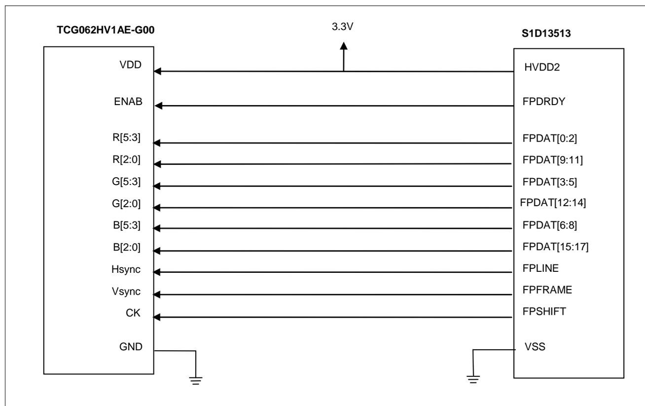
Figure 9-1 Connecting the TCG062HV1AE-G00 to the S1D13513
