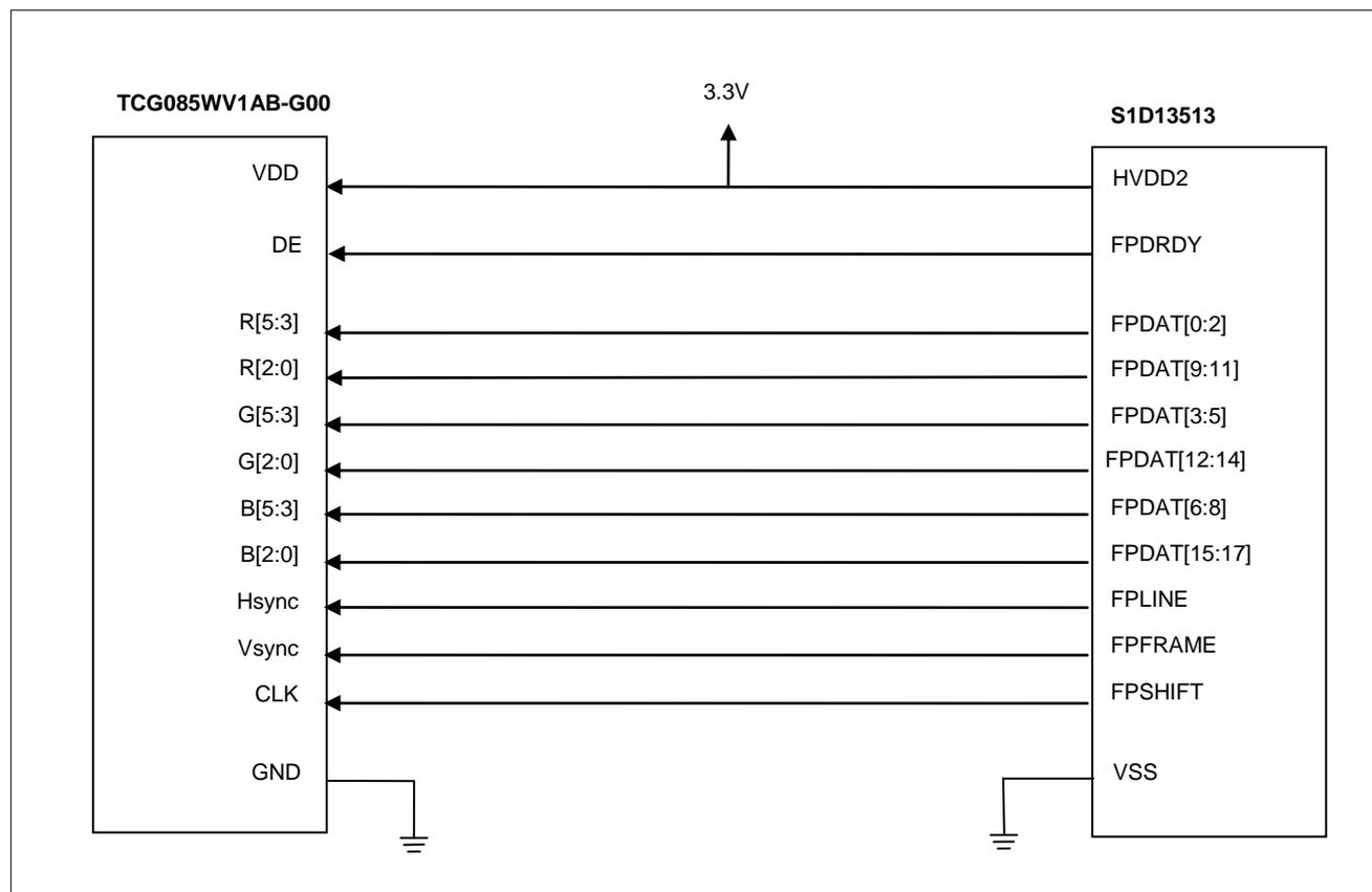
Figure 12-1 Connecting the TCG085WV1AB-G00 to the S1D13513
