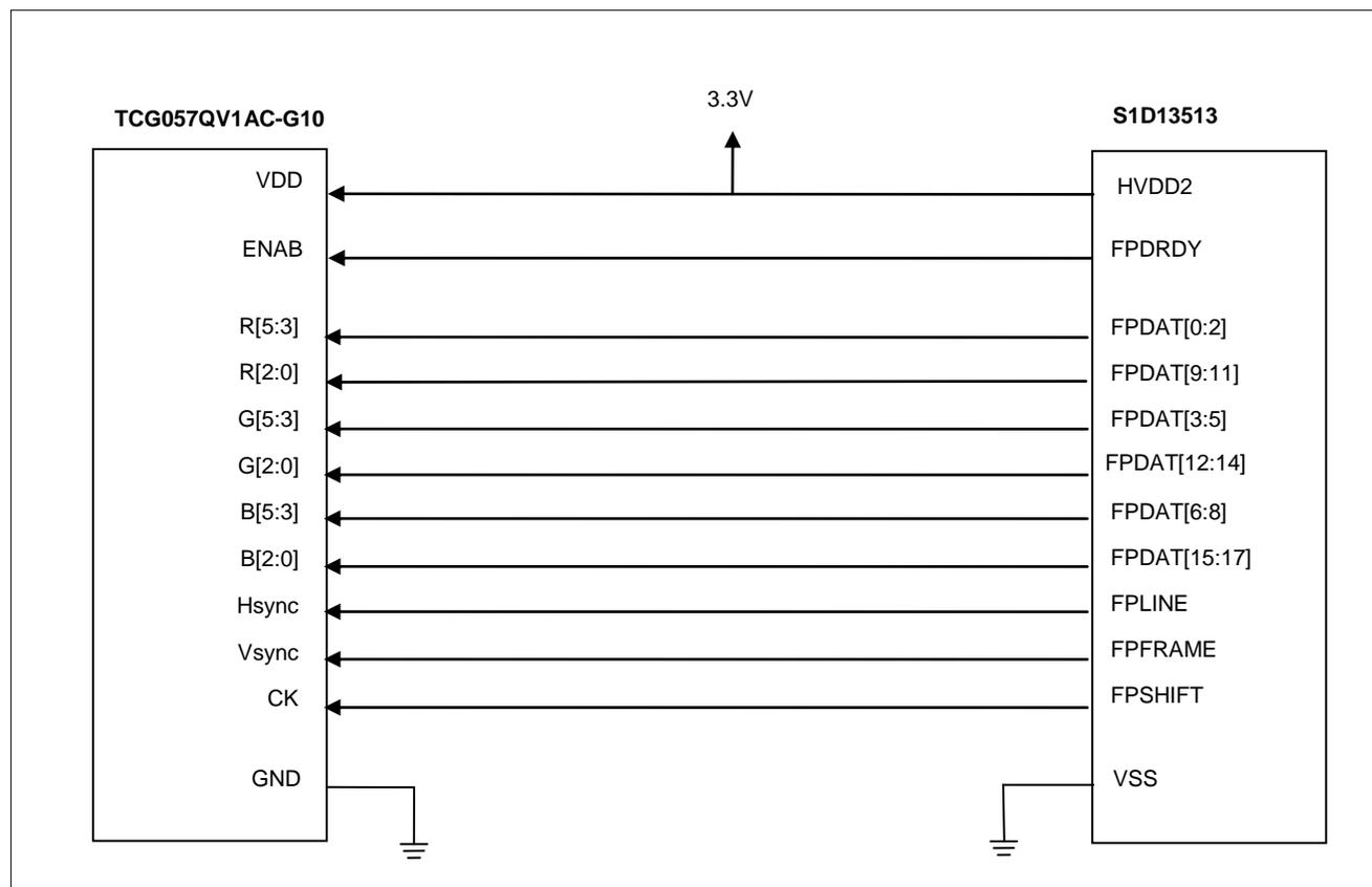
Figure 5-1 Connecting the TCG057QV1AC-G10 to the S1D13513
