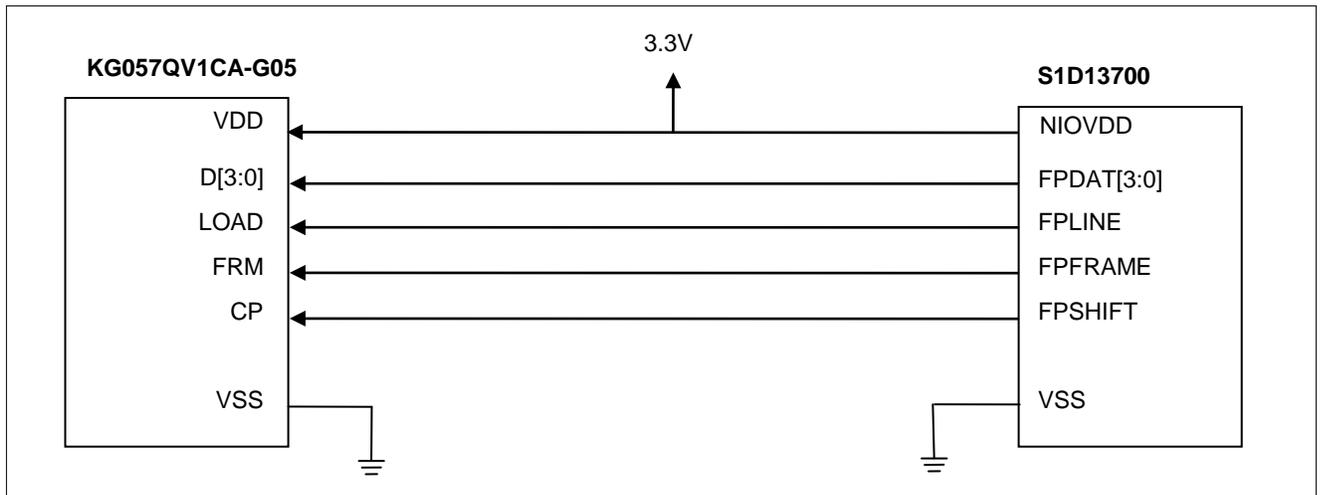
Figure 4-1 Connecting the KG057QV1CA-G05 to the S1D13700
