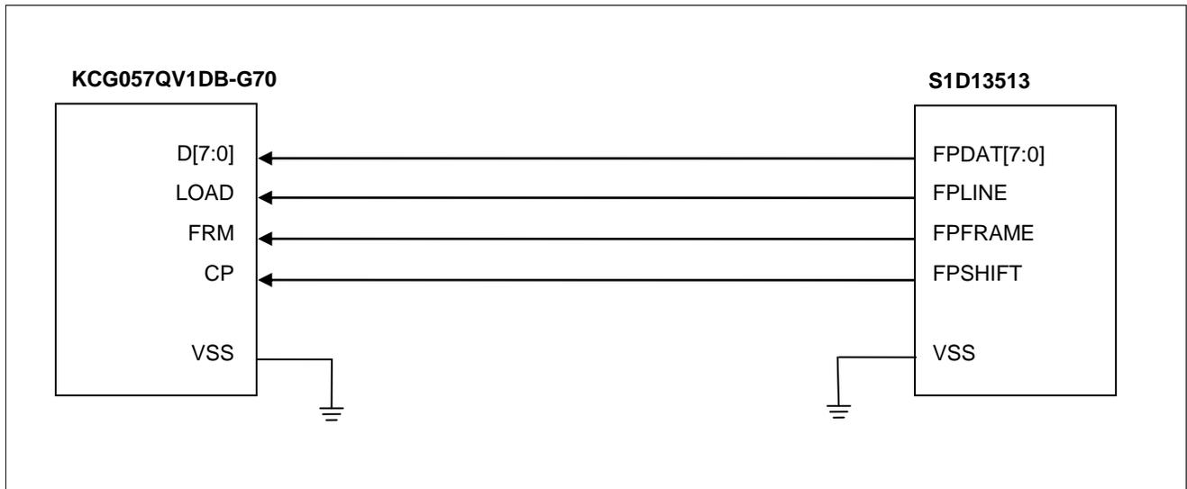
Figure 3-1 Connecting the KCG057QV1DB-G70 Panel to the S1D13513
