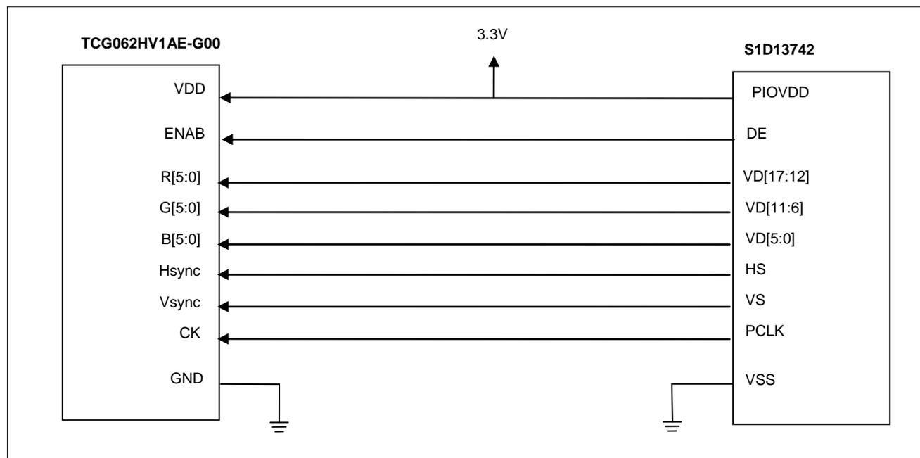
Figure 9-2 Connecting the TCG062HV1AE-G00 to the S1D13742
