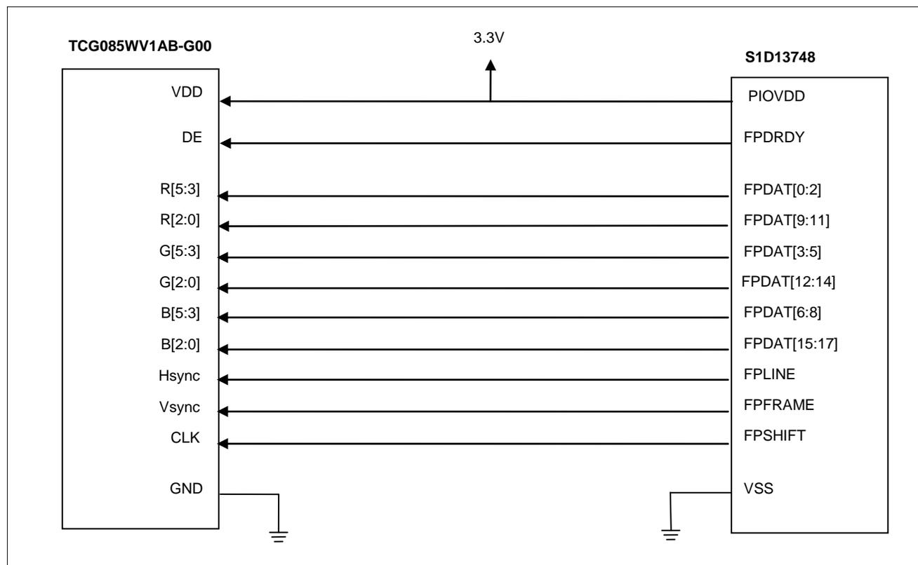
Figure 12-3 Connecting the TCG085WV1AB-G00 to the S1D13748
