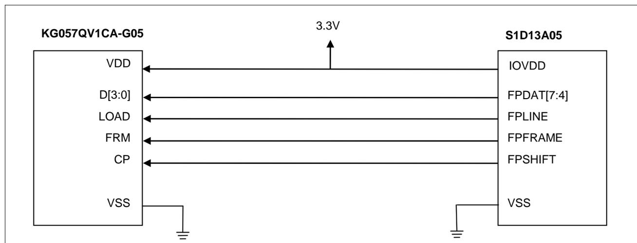
Figure 4-3 Connecting the KG057QV1CA-G05 to the S1D13A05
