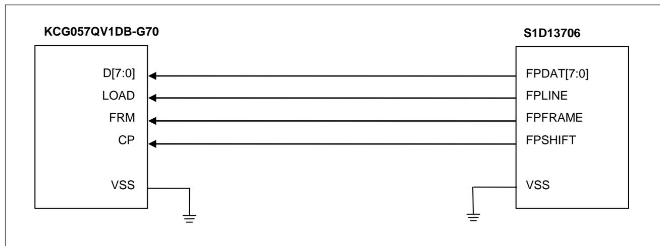
Figure 3-2 Connecting the KCG057QV1DB-G70 to the S1D13706
