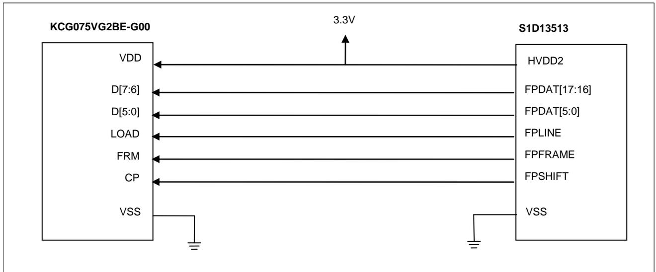
Figure 10-1 Connecting the KCG075VG2BE-G00 to the S1D13513
