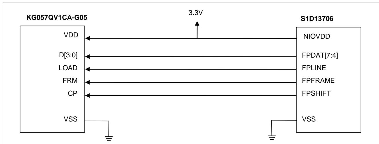
Figure 4-2 Connecting the KG057QV1CA-G05 to the S1D13706
