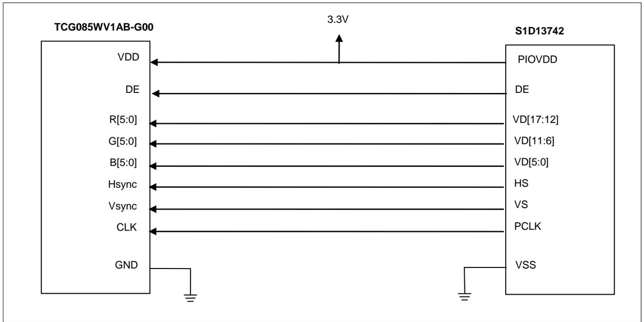
Figure 12-2 Connecting the TCG085WV1AB-G00 to the S1D13742
