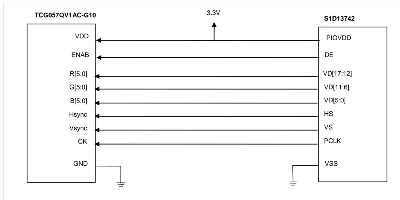
Figure 5-3 Connecting the TCG057QV1AC-G10 to the S1D13742
