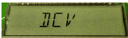
Figure 3.2.1-1 LCD screen when switched to DC voltage measurement
