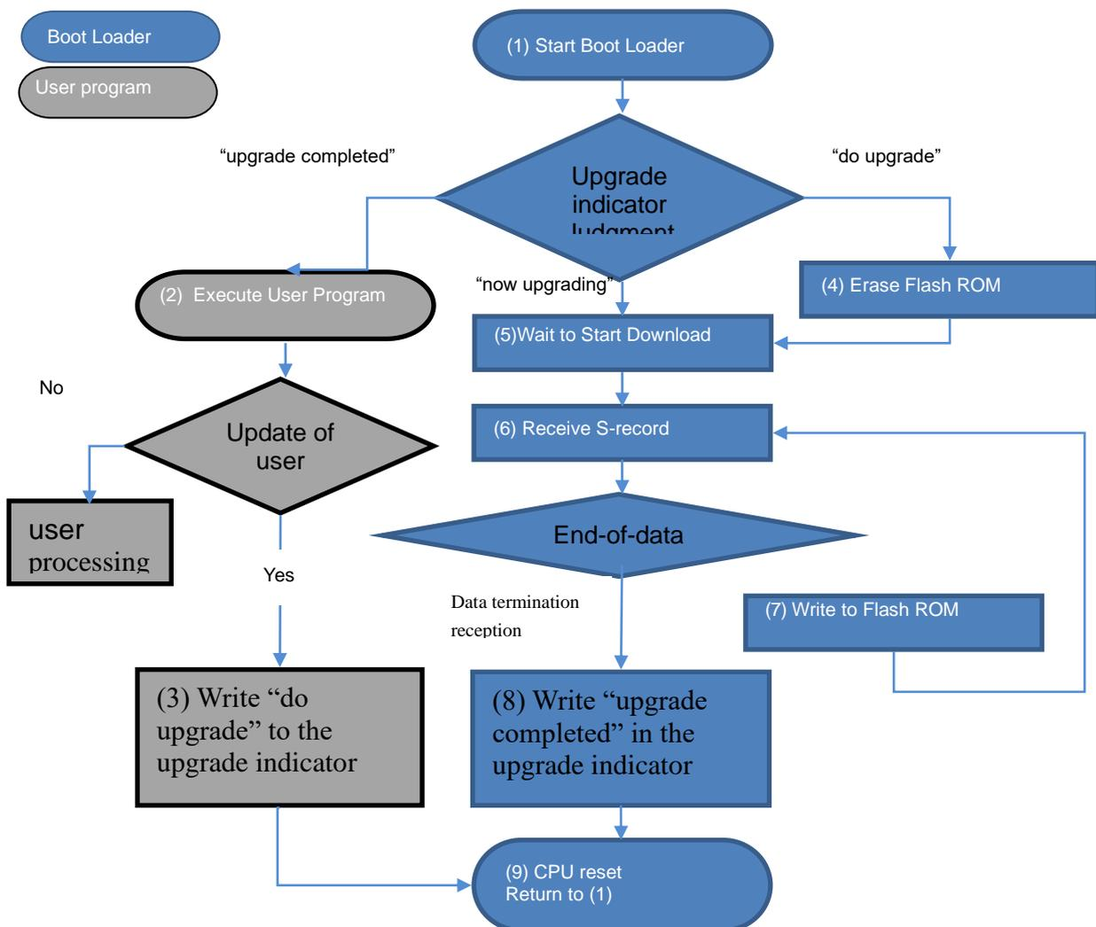
Figure 3.1.3.1 Boot loader operation flow
