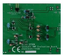
Figure 1.1 S5U1C31D51T2 External View
