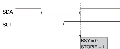
Figure 13.5.1 START/STOP Condition Interrupt Timings
