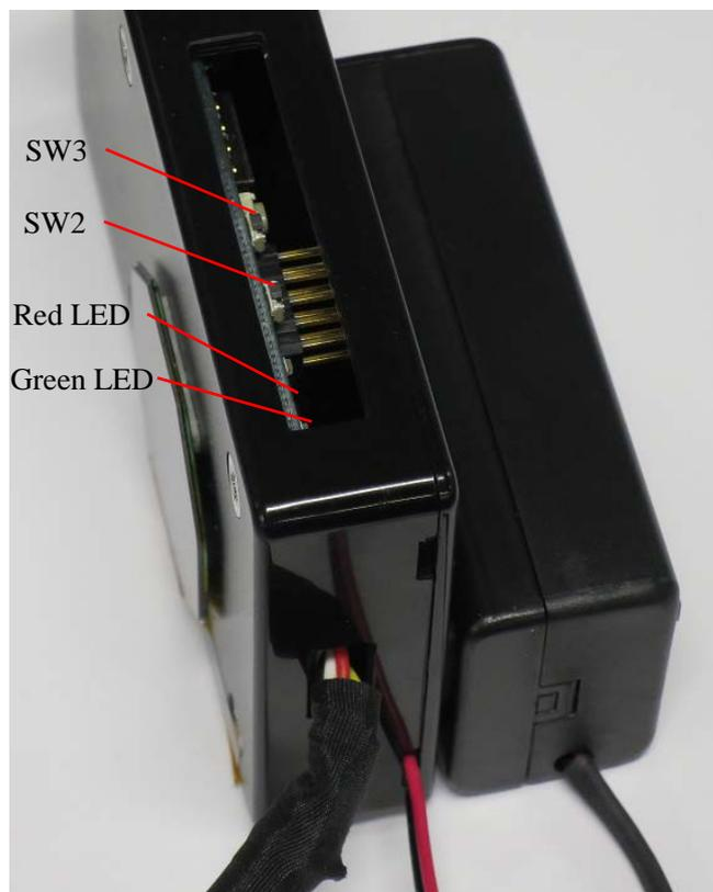
Figure 2-1 Push Switch and LED
