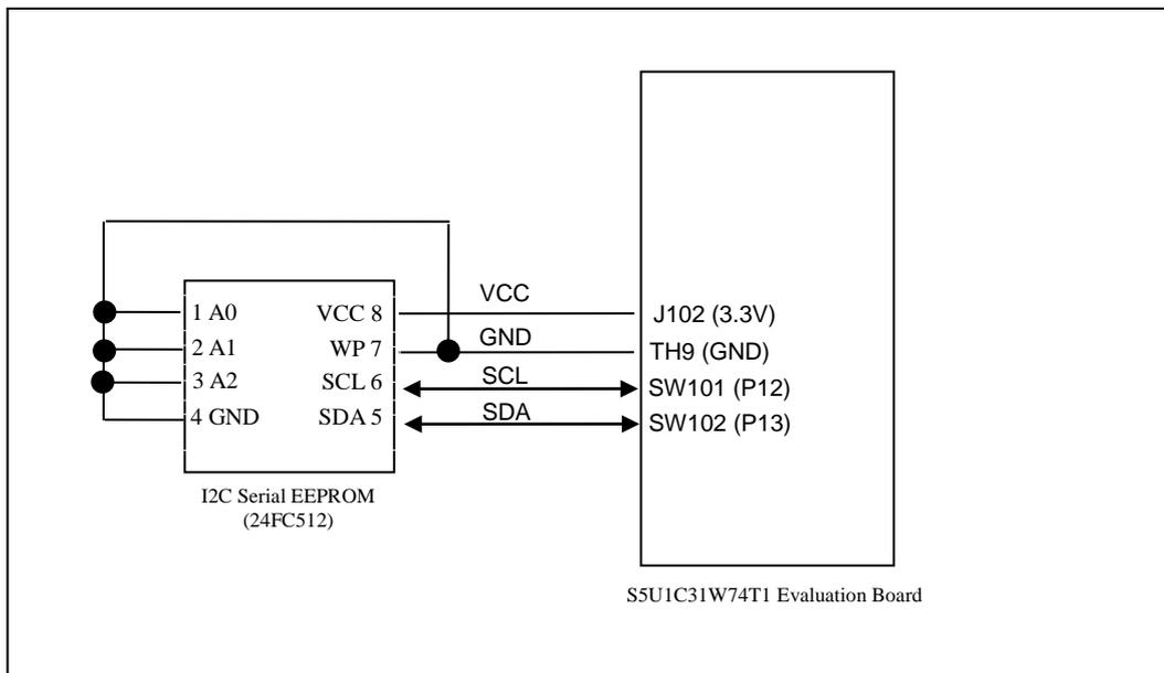
Figure 2.2.3.2 I2C Serial EEPROM Wiring to S5U1C31W74T1 Evaluation Board
