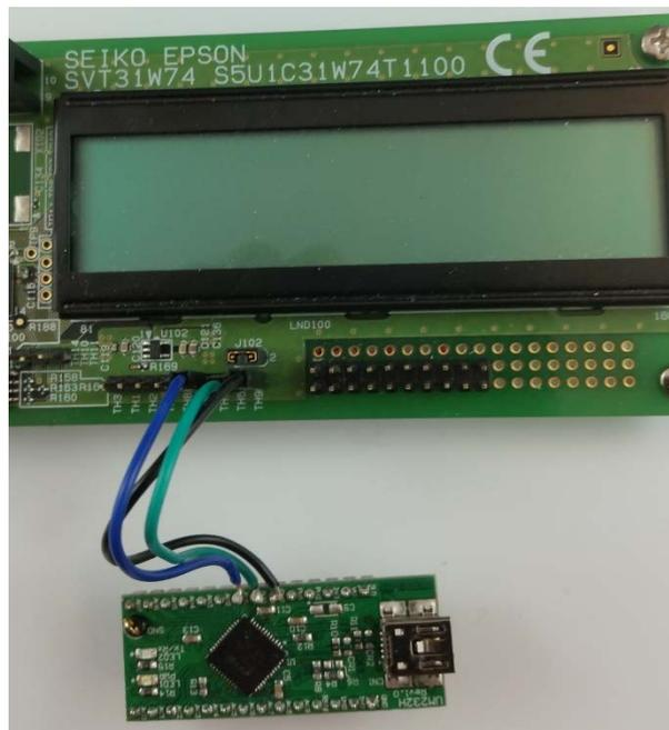
Figure 2.2.2.1 USB UART Board Connection to S5U1C31W74T1 Evaluation Board
