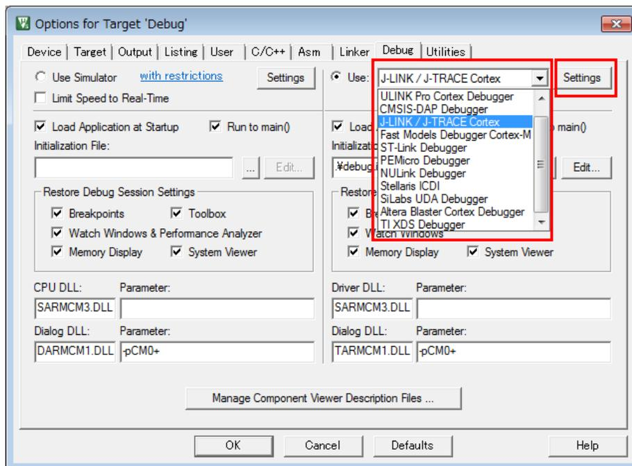
Figure 2.4.4.1 Debug Probe Selecting
