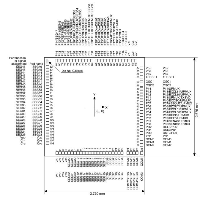
Pad opening No. 1–28, 55–81:  $X = 68 \mu m$ ,  $Y = 80 \mu m$ No. 29–54, 82–108:  $X = 80 \mu m$ ,  $Y = 68 \mu m$
