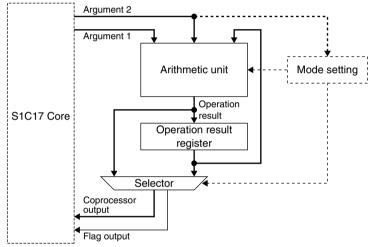
Figure 21.1.1 Multiplier/Divider Block Diagram
