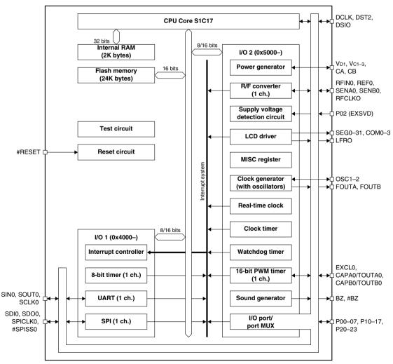
Figure 1.2.1 S1C17656 Block Diagram
