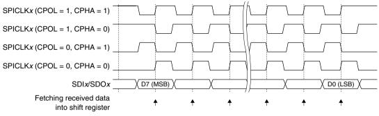
Figure 15.4.1 Clock and Data Transfer Timing
