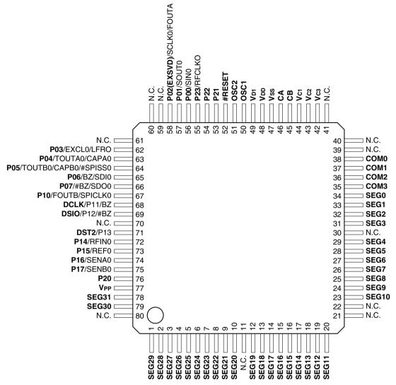
Figure 1.3.1.2 S1C17656 Pin Configuration Diagram (TQFP14-80pin)
