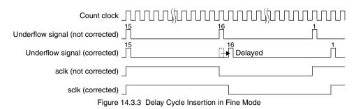
At initial reset, FMD[3:0] is set to 0x0, preventing insertion of delay cycles.
