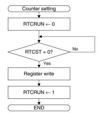
Figure 8.3.4.1 Procedure for Setting Counters
