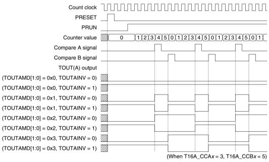
Figure 11.6.2 TOUT Output Waveform
