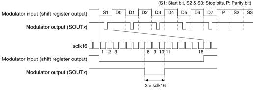
Figure 14.8.1 Transmission Signal Waveform
