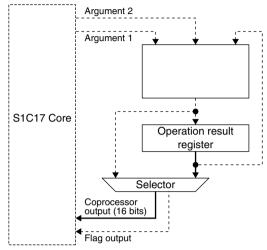
Figure 21.6.1 Data Path in Operation Result Read Mode
