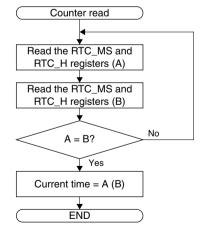
Figure 8.3.5.1 Procedure for Reading Counters
