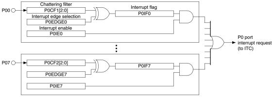
Figure 9.5.1 Port Input Interrupt Circuit Configuration
