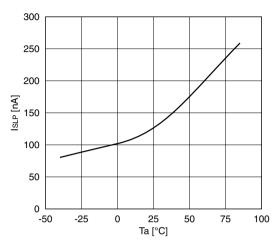
Current consumption-temperature characteristic during execution with OSC1A + clock gear OSC1A = 32.768kHz crystal, OSC3B = OFF,
