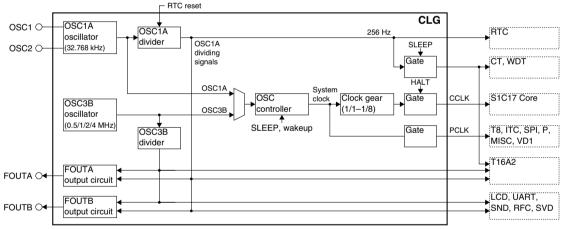
Figure 7.1.1 CLG Module Configuration
