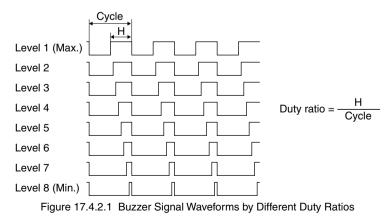
Note: BZDT[2:0] is ineffective in envelope mode, as the duty ratio is automatically controlled by the hardware.
