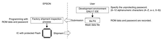
Figure 20.4.1 Shipment of IC with ROM Data Programmed and Flash Security Function Setting Flow
