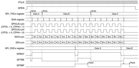
Figure 15.5.2 Data Transmission/Receiving Timing Chart (MSB first)
