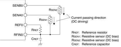
Figure 19.4.1.1 Connection Example in DC Oscillation Mode for Measuring Resistive Sensors
