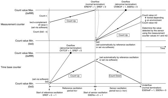
Figure 19.6.2.1 Counter Operations During Reference/Sensor Oscillation
