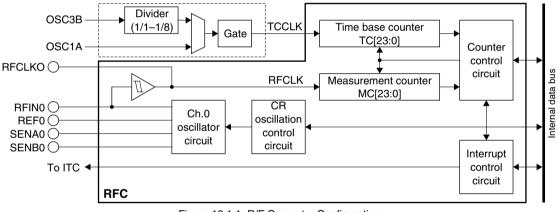
Figure 19.1.1 R/F Converter Configuration
