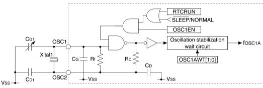
Figure 7.3.2.1 OSC1A Oscillator Circuit
