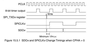
The half SPICLK*x* cycle will be secured from change of data to change of the clock for the second and following transmit data bits and the second and following bytes during continuous transfer.
