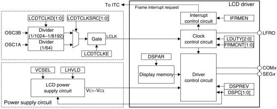
Figure 16.1.1 LCD Driver and Driver Power Supply Configuration
