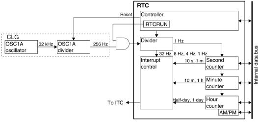
Figure 8.1.1 RTC Block Diagram
