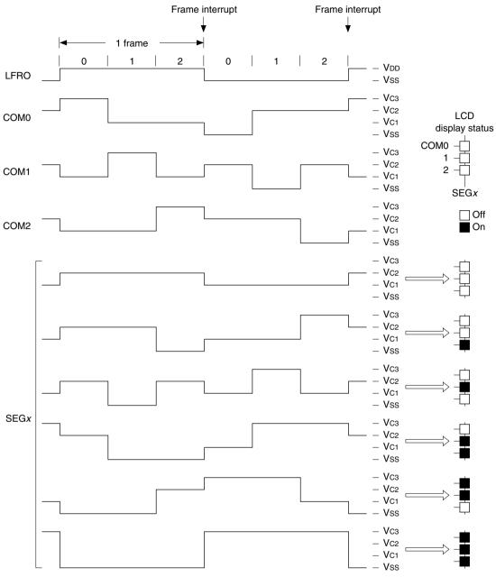
Figure 16.4.2.2 1/3 Duty Drive Waveform
