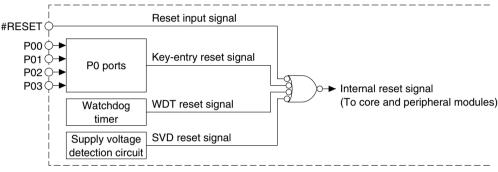
Figure 5.1.1 Configuration of Initial Reset Circuit
