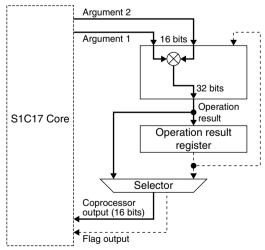
Figure 21.3.1 Data Path in Multiplication Mode
