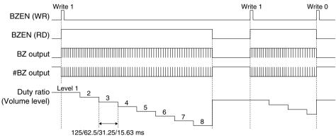
Figure 17.5.4.1 Buzzer Output in Envelope Mode
