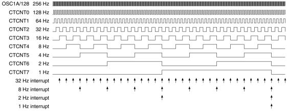
Figure 12.4.1 Clock Timer Timing Chart
