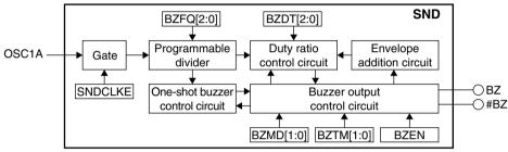
Figure 17.1.1 SND Module Configuration
