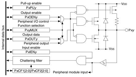
Figure 9.1.1 I/O Port Configuration
