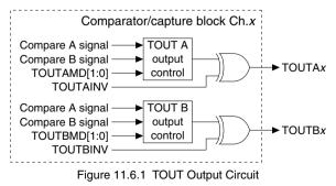
T16A2 includes two TOUT output circuits and their signal generation and output can be controlled individually. Although the output circuit and register names use letters 'A' and 'B' to distinguish two systems, it does not mean that they correspond to compare A and B signals.
