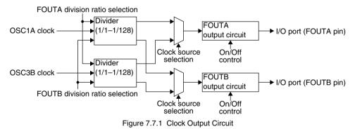
There are two output systems available: FOUTA and FOUTB. The FOUTA and FOUTB output circuits have the same functions.
