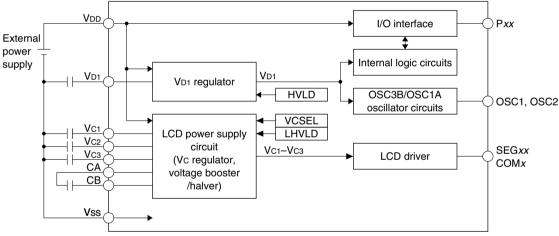
Figure 4.3.1 Configuration of Internal Power Supply Circuit
