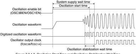
Figure 7.3.1.2 Oscillation Start Time and Oscillation Stabilization Wait Time
