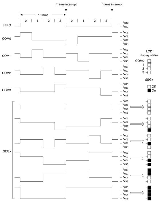
Figure 16.4.2.1 1/4 Duty Drive Waveform
