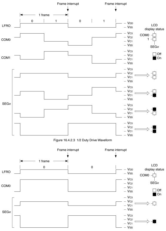
Figure 16.4.2.4 Static Drive Waveform
