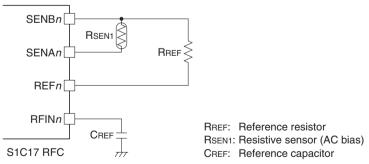
Figure 19.2.2.2 Connection Example in Resistive Sensor AC Oscillation Mode
