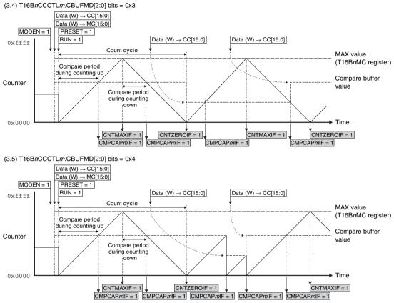
(Note that the T16BnINTF.CMPCAPmIF/CNTMAXIF/CNTZEROIF bit clearing operations via software are omitted from the figure.) Figure 15.4.3.2 Compare Buffer Operations
