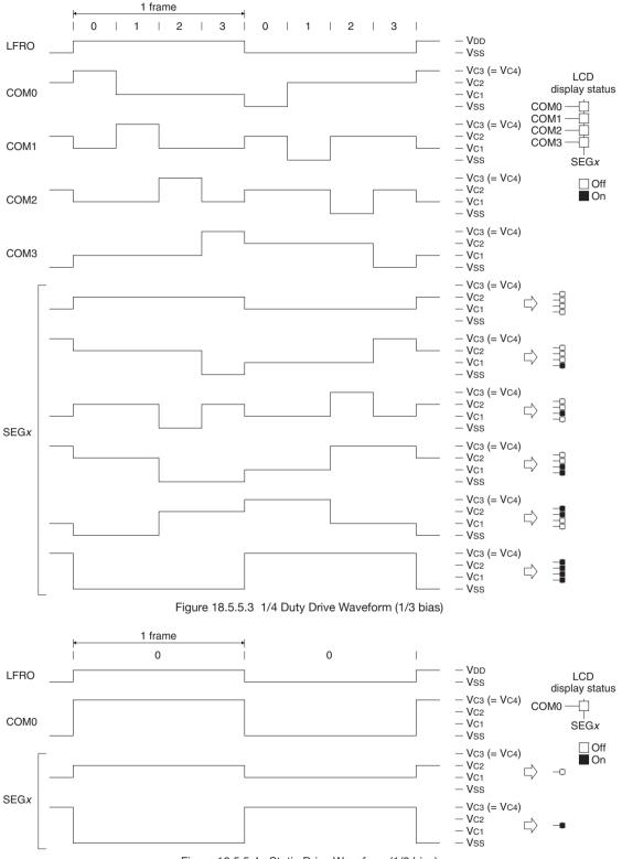
Figure 18.5.5.4 Static Drive Waveform (1/3 bias)
