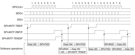
Figure 13.5.3.1 Example of Data Receiving Operations in Master Mode (SPInMOD.CHLN[3:0] bits = 0x7)
