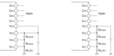
When 1/3 bias is selected (LCD24PWR.BISEL bit = 0) When 1/4 bias is selected (LCD24PWR.BISEL bit = 1) Figure 18.4.2.1 External Connection Example for External Voltage Application Mode 1 (resistor divider)
