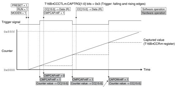
An overwrite error occurs as the T16BnINTF.CMPCAPmIF bit has not been cleared.
