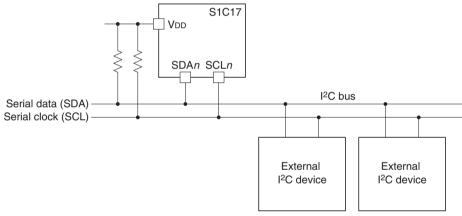
Figure 14.2.2.1 Connections between I2C and External I<sup>2</sup>C Devices
