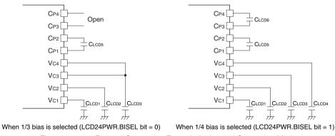
Figure 18.4.1.1 External Connection Example for Internal Generation Mode
