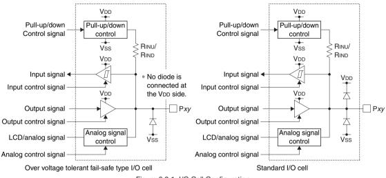
Figure 6.2.1 I/O Cell Configuration
