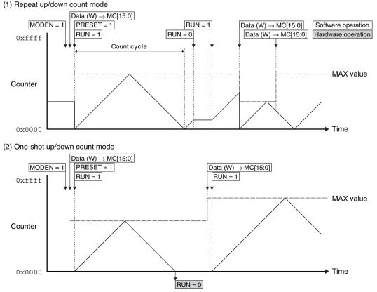
Figure 15.4.2.3 Operations in Repeat Up/Down Count and One-shot Up/Down Count Modes
