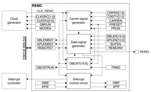
Figure 17.1.1 REMC Configuration
