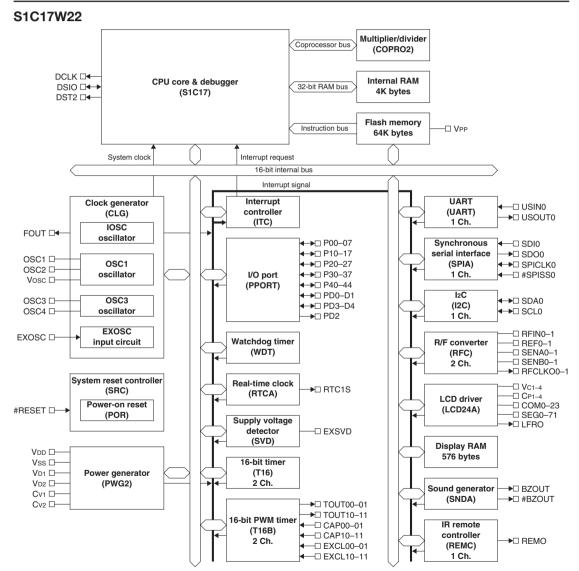
Figure 1.2.1 S1C17W22 Block Diagram
