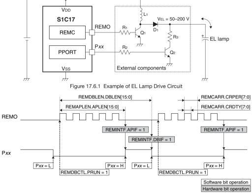
Figure 17.6.2 Example of Generated Drive Waveform
