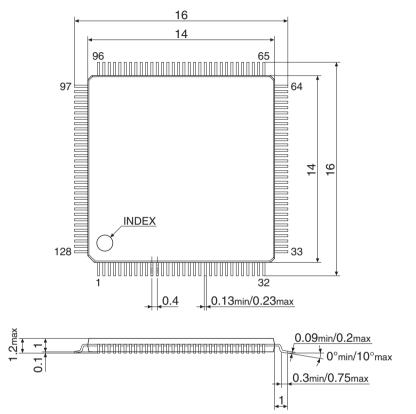
Figure 25.1 TQFP15-128PIN Package Dimensions
