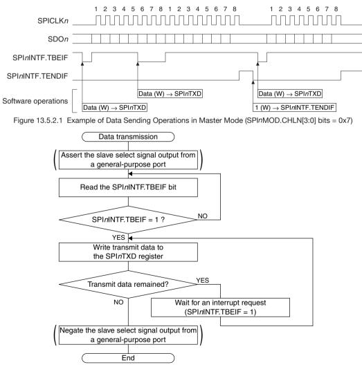
Figure 13.5.2.2 Data Transmission Flowchart in Master Mode
