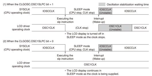
Figure 2.3.4.3 Clock Control Example in SLEEP Mode
