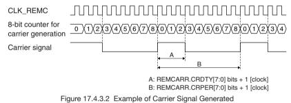
The carrier signal frequency and duty ratio can be calculated by the equations shown below.
