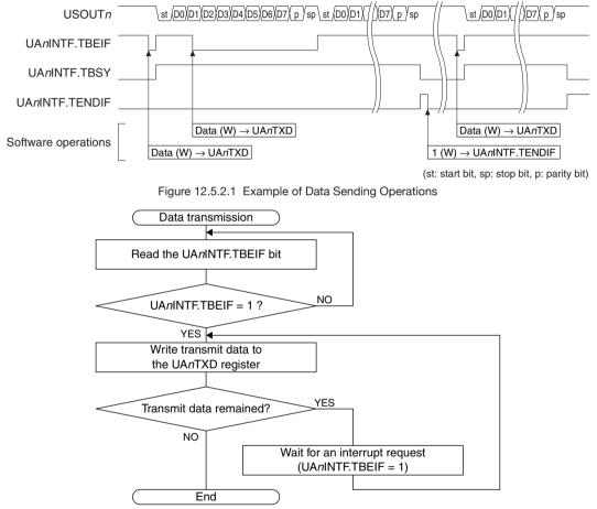
Figure 12.5.2.2 Data Transmission Flowchart
