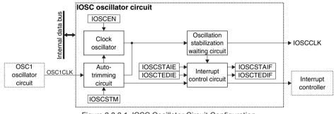
Figure 2.3.3.1 IOSC Oscillator Circuit Configuration
