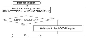
Figure 14.4.5.2 Slave Mode Data Transmission Flowchart
