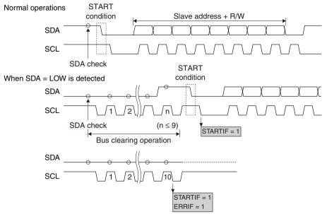
Figure 14.4.8.1 Automatic Bus Clearing Operation
