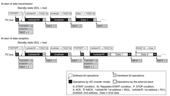
Figure 14.4.4.2 Example of Data Transfer Starting Operations in 10-bit Address Mode (Master Mode)
