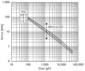
RFC reference/sensor oscillation current consumption-frequency characteristic
