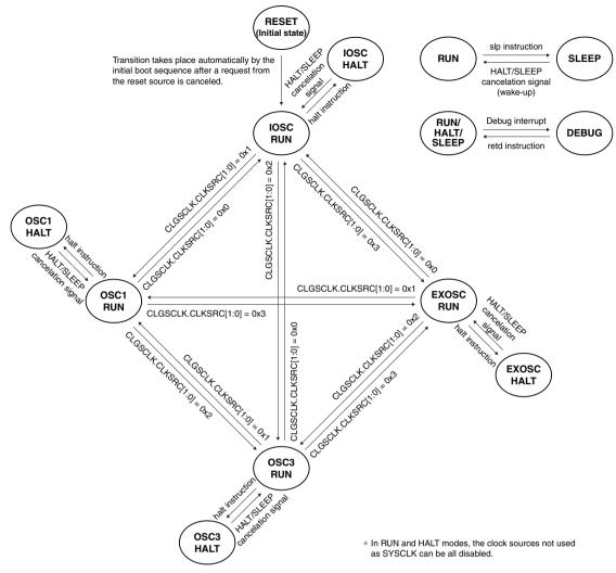
Figure 2.4.2.1 Operating Mode-to-Mode State Transition Diagram
