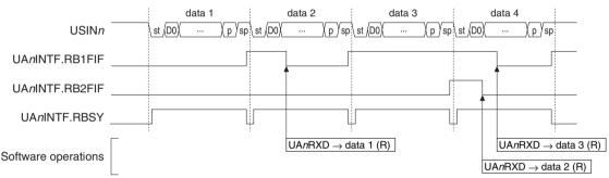
(st: start bit, sp: stop bit, p: parity bit)
