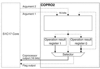
Figure 22.6.1 Data Path in Operation Result Read Mode
