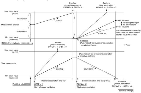
Figure 19.4.4.1 Counter Operations During Reference/Sensor Oscillation
