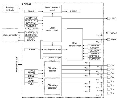
Figure 18.1.1 LCD24A Configuration
