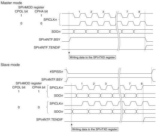
Figure 13.6.1 SPInINTF.BSY and SPInINTF.TENDIF Bit Set Timings (when SPInMOD.CHLN[3:0] bits = 0x7)
