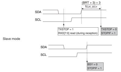
(fcLK\_l2Cn: I2C operating clock frequency [Hz], BRT: I2CnBR.BRT[6:0] bits setting value (1 to 127)) Figure 14.5.1 START/STOP Condition Interrupt Timings
