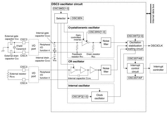
Figure 2.3.3.3 OSC3 Oscillator Circuit Configuration
