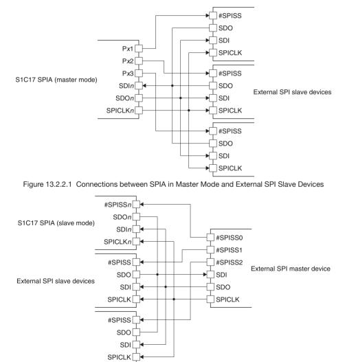
Figure 13.2.2.2 Connections between SPIA in Slave Mode and External SPI Master Device
