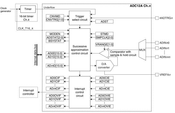
Figure 20.1.1 ADC12A Configuration
