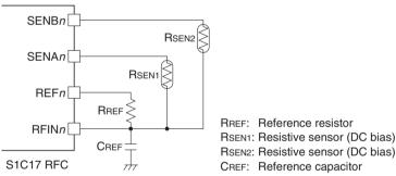
\* Leave the unused pin (SENAn or SENBn) open if one resistive sensor only is used. Figure 19.2.2.1 Connection Example in Resistive Sensor DC Oscillation Mode
