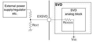
Figure 10.2.2.1 Connection between EXSVD Pin and External Power Supply
