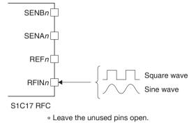
Figure 19.2.2.3 External Clock Input in External Clock Input Mode
