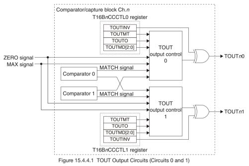
Each timer channel includes two (four, or six) TOUT output circuits and their signal generation and output can be controlled individually.
