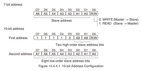
The following shows a procedure to start data transfer in 10-bit address mode when the I2C Ch.*n* is placed into master mode (see the 7-bit mode descriptions above for control procedures when a NACK is received or sending/ receiving data). Figure 14.4.4.2 shows an operation example.
