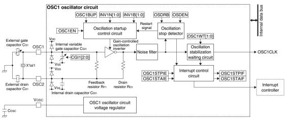
Figure 2.3.3.2 OSC1 Oscillator Circuit Configuration
