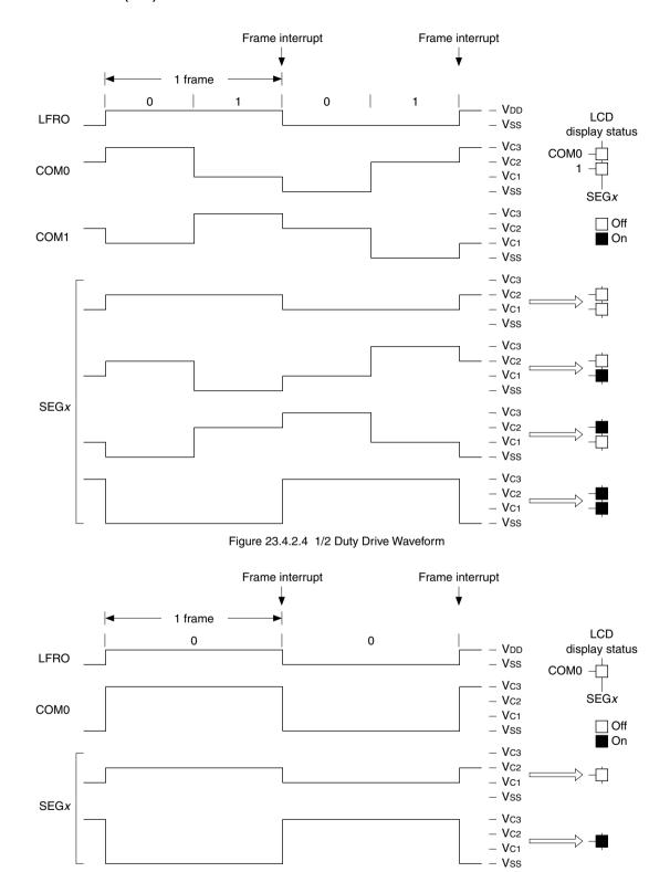
Figure 23.4.2.5 Static Drive Waveform
