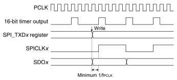
Figure 19.5.1 SDOx and SPICLKx Change Timings when CPHA = 0
