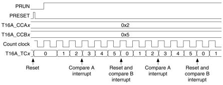
Figure 13.5.4.1 Operation Timing in Comparator Mode
