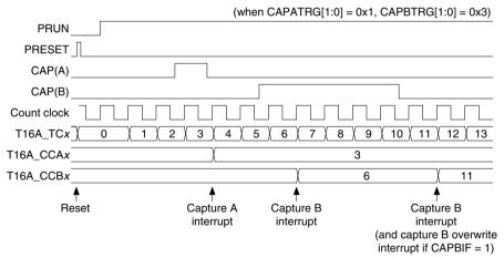
Figure 13.5.4.2 Operation Timing in Capture Mode
