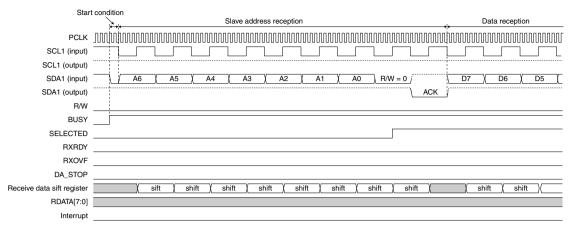
Figure 21.5.7 I2CS Timing Chart 3 (start condition → data reception)
