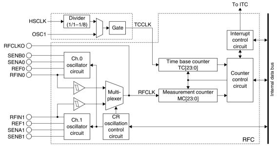
Figure 25.1.1 R/F Converter Configuration
