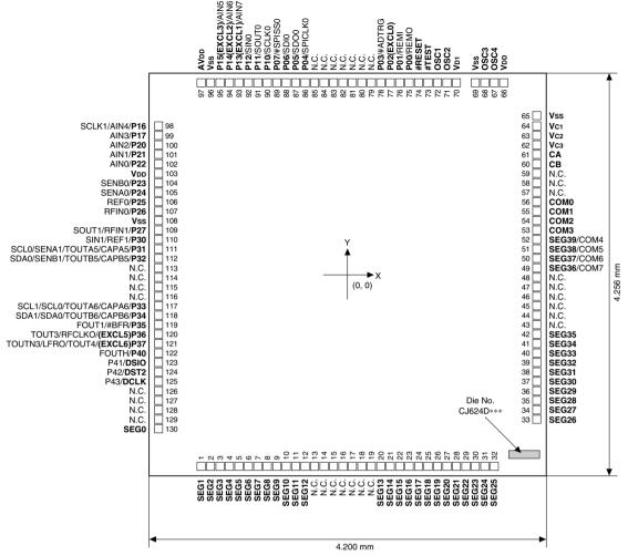
Figure 1.3.2.2 S1C17604 Pad Configuration Diagram
