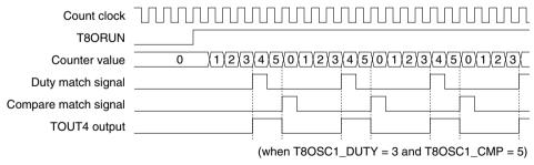
Figure 14.8.1 PWM Output Waveform
