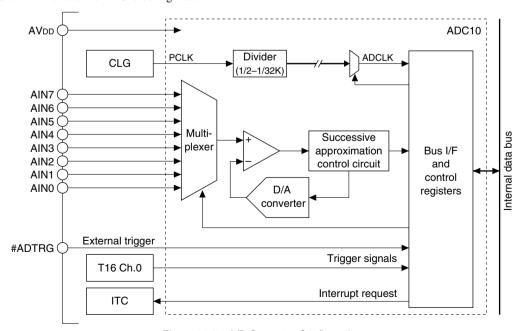
Figure 24.1.1 A/D Converter Configuration
