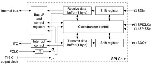
Figure 19.1.1 SPI Module Configuration
