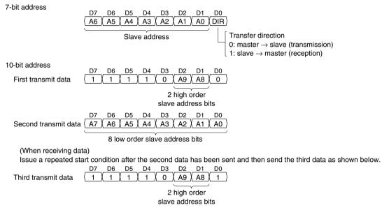
Figure 20.5.2 Transmit Data Specifying Slave Address and Transfer Direction
