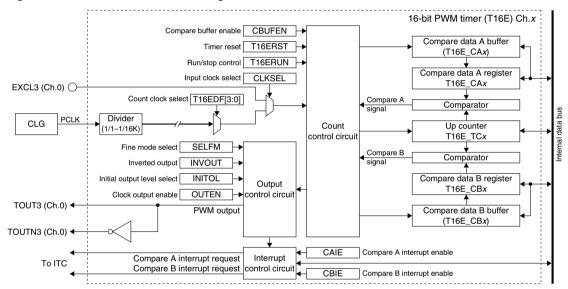
Figure 12.1.1 T16E Module Configuration
