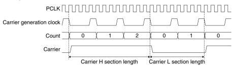
Figure 22.7.1 Carrier Signal Generation
