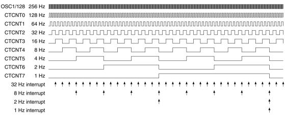
Figure 15.4.1 Clock Timer Timing Chart
