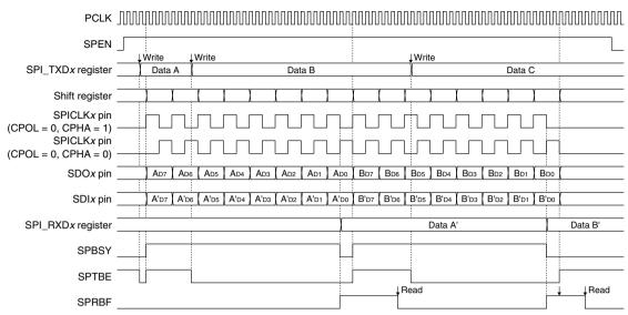
Figure 19.5.2 Data Transmission/Receiving Timing Chart (MSB first)
