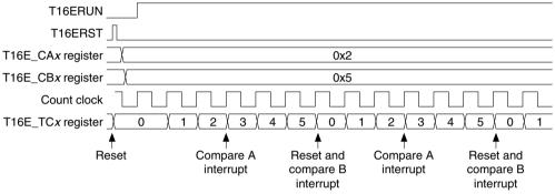
Figure 12.6.1 Basic Counter Operation Timing
