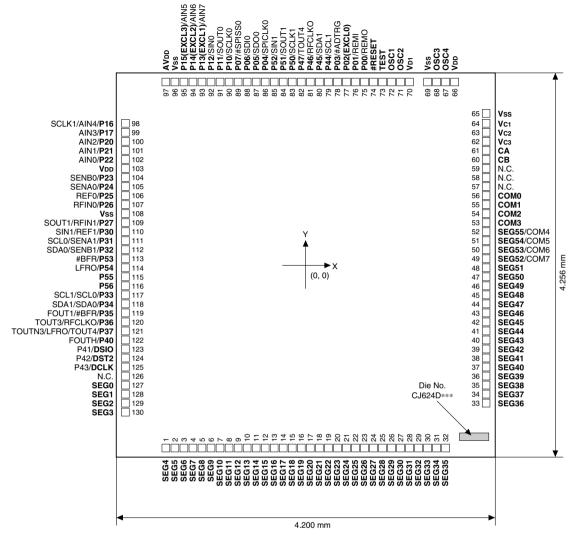
Figure 1.3.3.2 S1C17622 Pad Configuration Diagram
