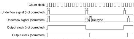
Figure 10.8.1 Delay Cycle Insertion in Fine Mode
