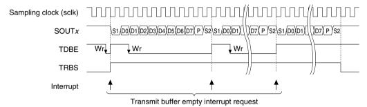
S1: Start bit, S2: Stop bit, P: Parity bit, Wr: Data write to transmit data buffer Figure 18.5.1 Data Transmission Timing Chart
