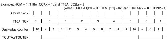
Figure 13.6.4 PWM Waveform Output Timings in Half Clock Mode
