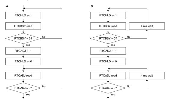
Figure 8.3.6.1 Procedure for Executing 30-second Correction
