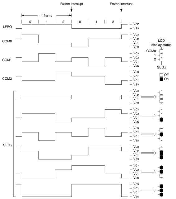
Figure 23.4.2.3 1/3 Duty Drive Waveform
