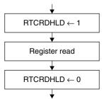
Figure 8.3.7.1 Procedure for Reading Counters
