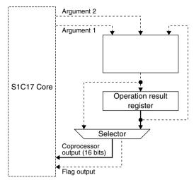
Figure 28.6.1 Data Path in Operation Result Read Mode
