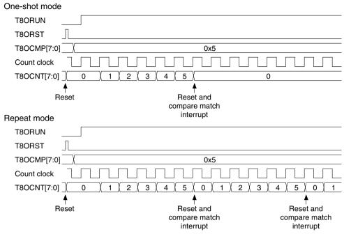
Figure 14.7.1 Basic Counter Operation Timing
