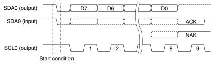
Figure 20.5.3 ACK and NAK
