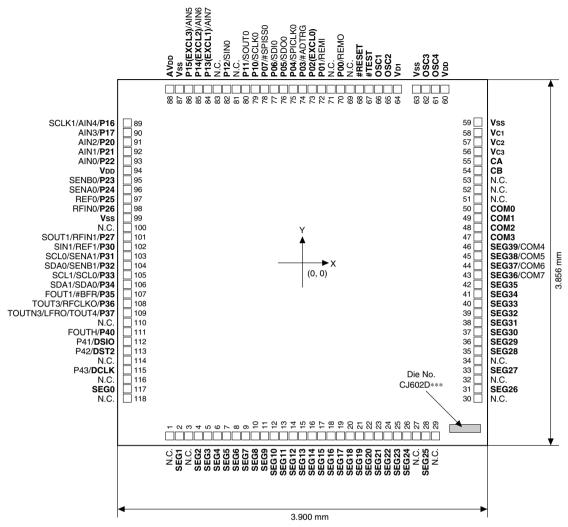
Figure 1.3.4.3 S1C17602/621 Pad Configuration Diagram
