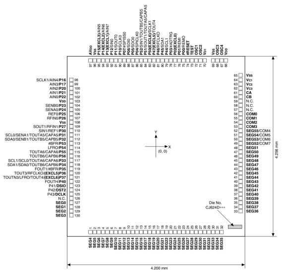
Figure 1.3.1.2 S1C17624 Pad Configuration Diagram
