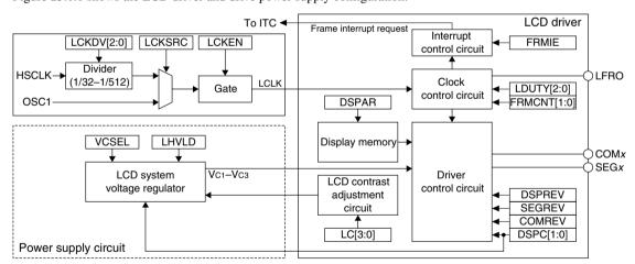
Figure 23.1.1 LCD Driver and Driver Power Supply Configuration
