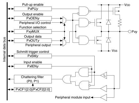
Figure 9.1.1 I/O Port Configuration
