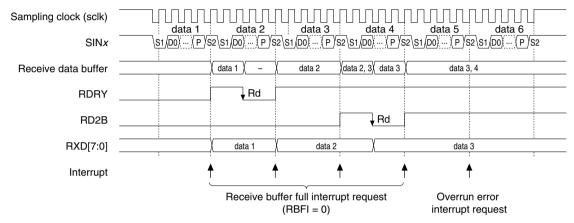
S1: Start bit, S2: Stop bit, P: Parity bit, Rd: Data read from RXD[7:0] Figure 18.5.2 Data Receiving Timing Chart
