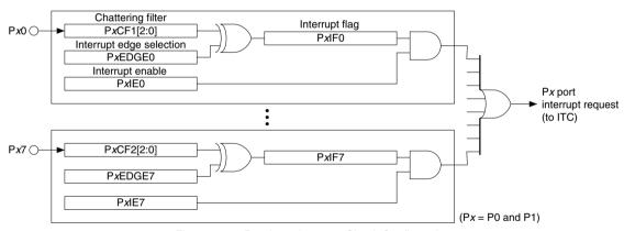
Figure 9.7.1 Port Input Interrupt Circuit Configuration
