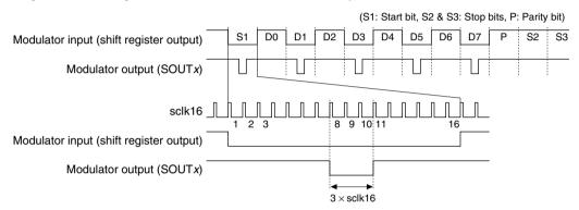
Figure 18.8.1 Transmission Signal Waveform
