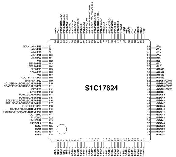
Figure 1.3.1.1 S1C17624 Pin Configuration Diagram (TQFP15-128pin)
