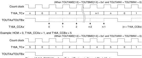
Figure 13.6.3 PWM Waveform Output Timings in Normal Clock Mode
