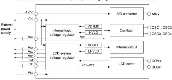
Figure 4.3.1 Configuration of Power Supply Circuit
