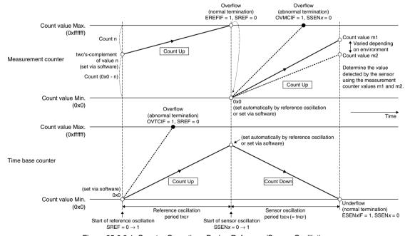
Figure 25.6.2.1 Counter Operations During Reference/Sensor Oscillation
