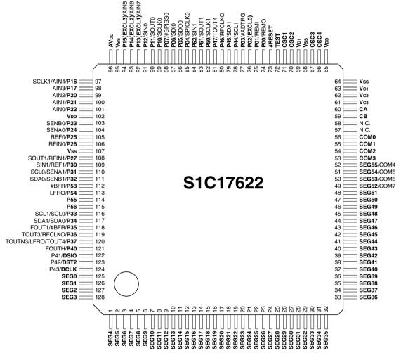
Figure 1.3.3.1 S1C17622 Pin Configuration Diagram (TQFP15-128pin)
