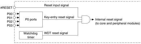
Figure 5.1.1 Configuration of Initial Reset Circuit
