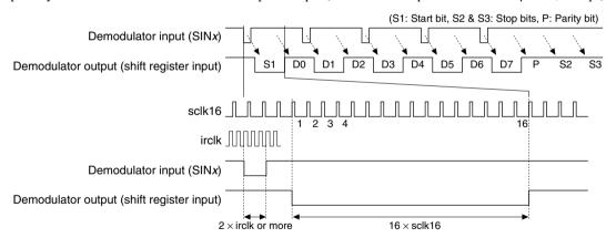
Figure 18.8.2 Receive Signal Waveform
