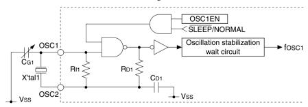
Figure 7.3.3.1 OSC1 Oscillator Circuit (S1C17622/602/621)
