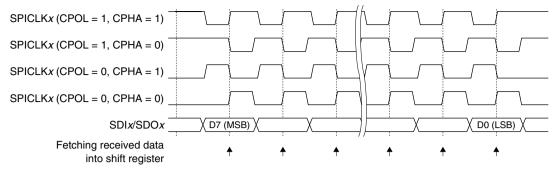
Figure 19.4.1 Clock and Data Transfer Timing
