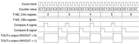
Figure 12.7.3 Fine Mode Clock Output
