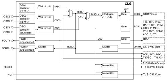
Figure 7.1.1 CLG Module Configuration
