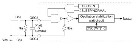
Figure 7.3.2.1 OSC3 Oscillator Circuit
