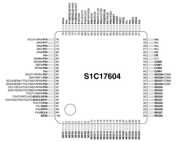
Figure 1.3.2.1 S1C17604 Pin Configuration Diagram (TQFP14-100pin)
