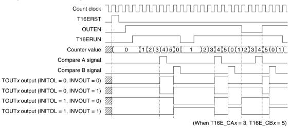
Figure 12.7.2 T16E Output Waveform
