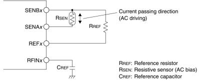
Figure 25.4.1.2 Connection Example in AC Oscillation Mode for Measuring Resistive Sensors
