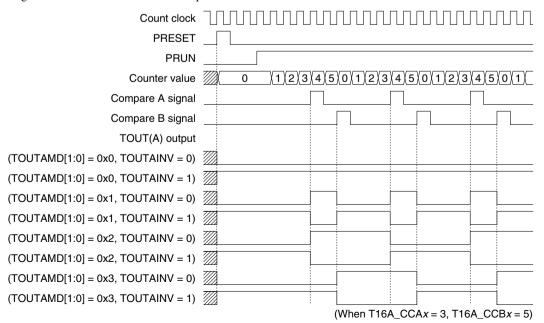
Figure 13.6.2 TOUT Output Waveform
