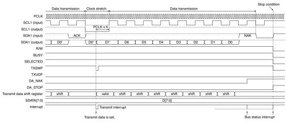
Figure 21.5.6 I2CS Timing Chart 2 (data transmission → stop condition)
