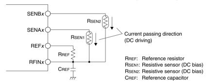
Figure 25.4.1.1 Connection Example in DC Oscillation Mode for Measuring Resistive Sensors
