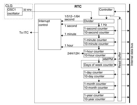
Figure 8.1.1 RTC Block Diagram
