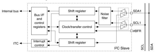
Figure 21.1.1 I2CS Module Configuration
