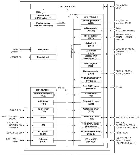
Figure 1.2.1 Block Diagram
