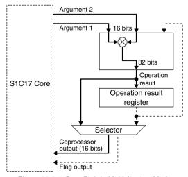
Figure 28.3.1 Data Path in Multiplication Mode
