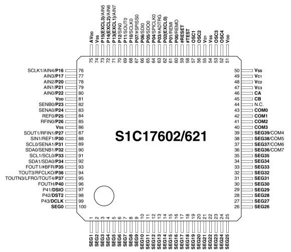
Figure 1.3.4.1 S1C17602/621 Pin Configuration Diagram (TQFP14-100pin)
