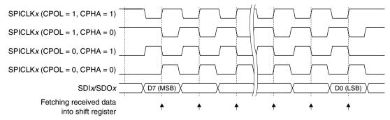
Figure 19.7.1 Clock and Data Transfer Timing
