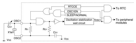
Figure 7.3.3.2 OSC1 Oscillator Circuit (S1C17624/604)
