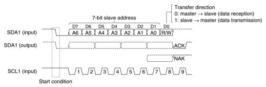
Figure 21.5.1 Receiving Slave Address and Data Direction Bit
