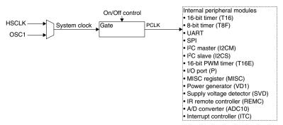
Figure 7.6.1 Peripheral Module Clock Control Circuit
