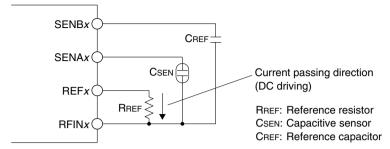
Figure 25.4.1.3 Connection Example in DC Oscillation Mode for Measuring Capacitive Sensors
