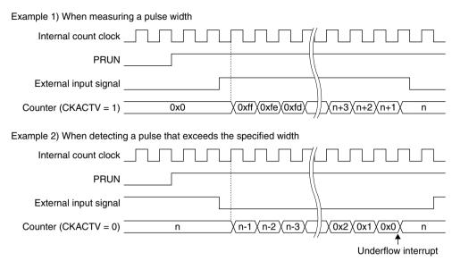
Figure 11.3.3.1 Count Operation in Pulse Width Measurement Mode
