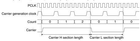
Figure 22.3.1 Carrier Signal Generation
