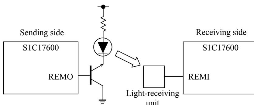
Figure 3.26 Remote controller (REMC) sample software's hardware connection diagram
