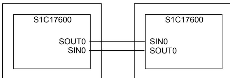
Figure 3.11 Sample software's hardware connection diagram for UART using OSC3
