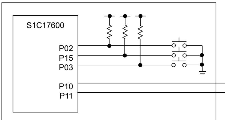
Figure 3.1 I/O ports (P) sample software's hardware connection diagram
