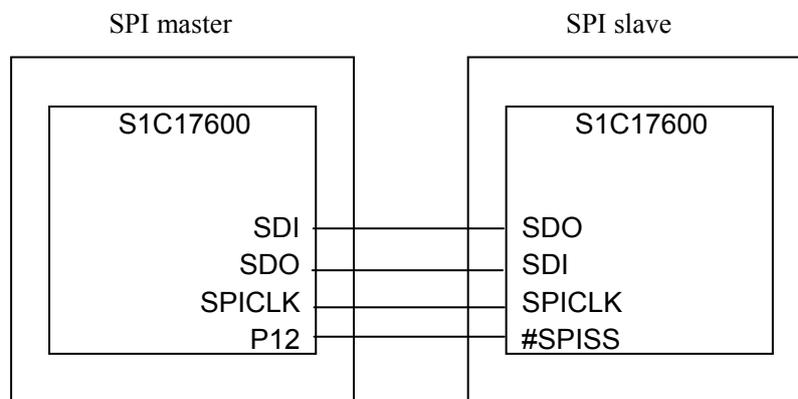
Figure 3.14 SPI master and slave sample software's hardware connection diagram
