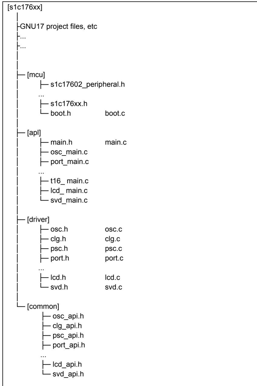
Figure 2.1 Block diagram for S1C17600 series sample software directories
