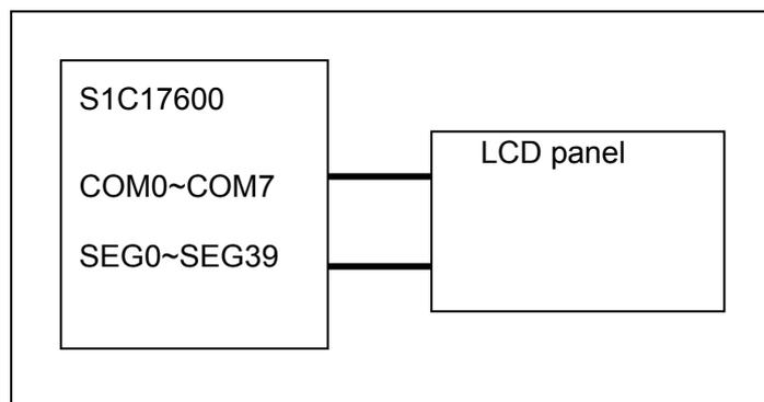
Figure 3.20 LCD driver (LCD) sample software's hardware connection diagram
