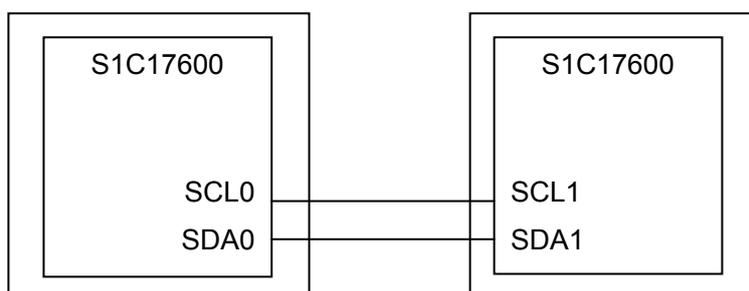
Figure 3.17 I2C master (I2CM) and slave (I2CS) sample software's hardware connection diagram
