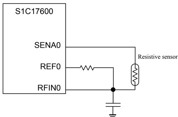
Figure 3.23 R/F converter (RFC) sample software's hardware connection diagram
