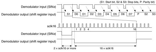
Figure 14.8.2 Receive Signal Waveform
