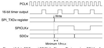
Figure 15.5.1 SDOx and SPICLKx Change Timings when CPHA = 0
