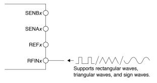
Figure 21.4.2.1 External Clock Input
