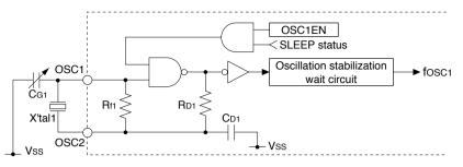
Figure 7.3.3.1 OSC1 Oscillator Circuit
