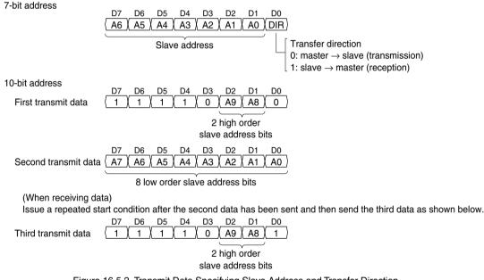
Figure 16.5.2 Transmit Data Specifying Slave Address and Transfer Direction
