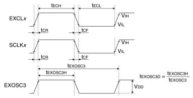
Figure 25.5.1 External Clock Input Timing
