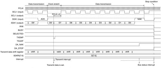
Figure 17.5.6 I2CS Timing Chart 2 (data transmission  $\rightarrow$  stop condition)
