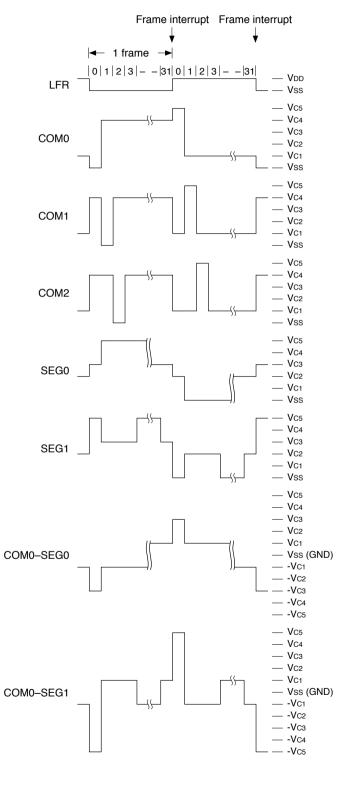
Figure 19.5.2.1 1/32 Duty Drive Waveform
