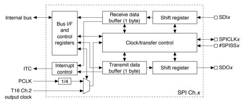
Figure 15.1.1 SPI Module Configuration (1 channel)
