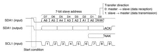
Figure 17.5.1 Receiving Slave Address and Data Direction Bit
