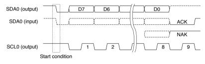
Figure 16.5.3 ACK and NAK
