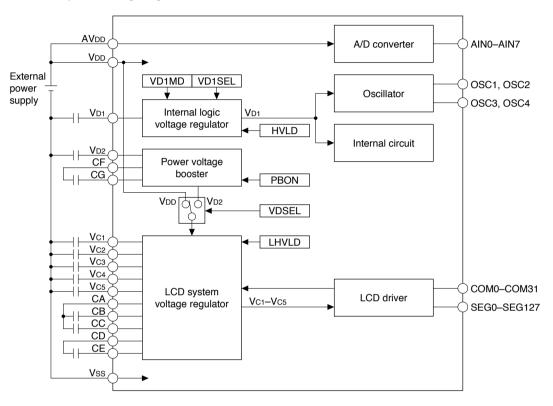
Figure 4.3.1 Configuration of Power Supply Circuit
