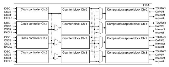
Figure 10.4.3.1 Timer Configuration in Normal Channel Mode (two comparator/capture blocks × four channels)
