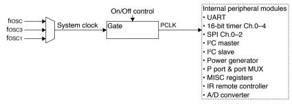
Figure 7.6.1 Peripheral Module Clock Control Circuit
