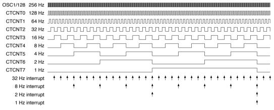
Figure 11.4.1 Clock Timer Timing Chart
