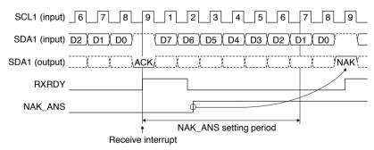
Figure 17.5.3 NAK\_ANS Setting and NAK Response Timing
