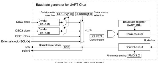
Figure 14.3.1 Baud Rate Generator
