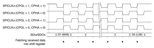
Figure 15.4.1 Clock and Data Transfer Timing
