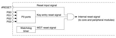
Figure 5.1.1 Configuration of Initial Reset Circuit
