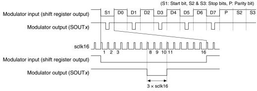
Figure 14.8.1 Transmission Signal Waveform
