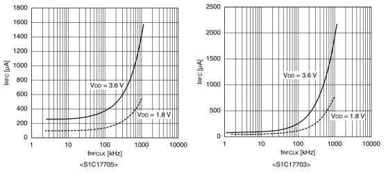
RFC reference/sensor oscillation current consumption-frequency characteristic (Capacitive sensor DC oscillation mode)
