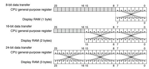
Figure 3.4.2.1 Data Transfer Between CPU General-Purpose Register and Display RAM (SRRVS = 1)
