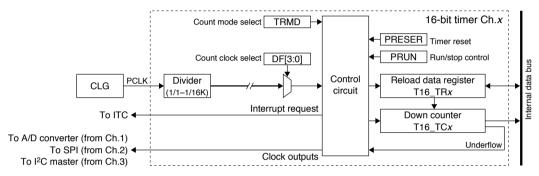
Figure 9.1.1 T16 Configuration (1 Channel)
