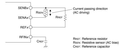
Figure 21.4.1.2 Connection Example in AC Oscillation Mode for Measuring Resistive Sensors
