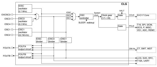
Figure 7.1.1 CLG Module Configuration
