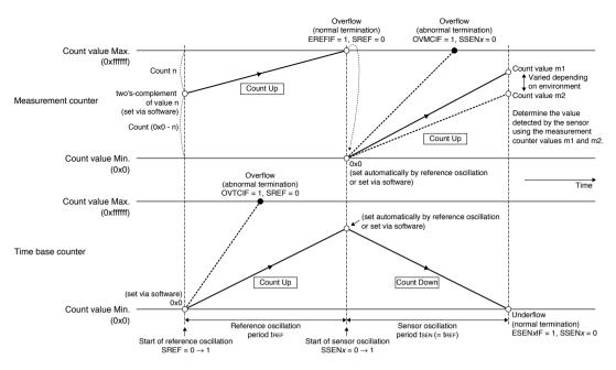
Figure 21.6.2.1 Counter Operations During Reference/Sensor Oscillation
