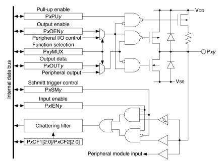
Figure 8.1.1 I/O Port Configuration
