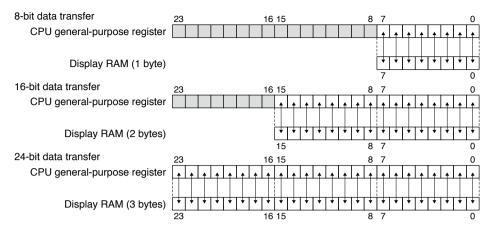
Figure 3.4.2.2 Data Transfer Between CPU General-Purpose Register and Display RAM (SRRVS = 0)
