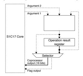
Figure 24.6.1 Data Path in Operation Result Read Mode
