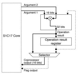
Figure 24.3.1 Data Path in Multiplication Mode
