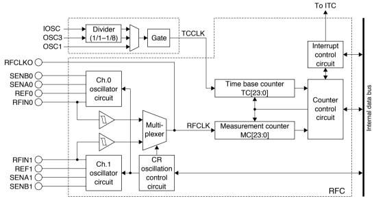
Figure 21.1.1 R/F Converter Configuration
