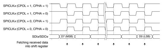
Figure 15.7.1 Clock and Data Transfer Timing
