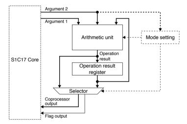
Figure 24.1.1 Multiplier/Divider Block Diagram
