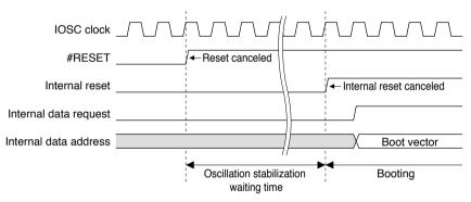
Figure 5.2.1 Operation Sequence Following Cancellation of Initial Reset
