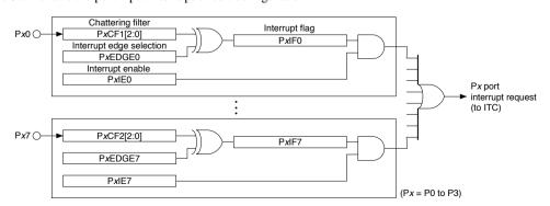
Figure 8.7.1 Port Input Interrupt Circuit Configuration
