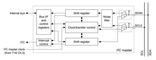
Figure 16.1.1 I2CM Module Configuration
