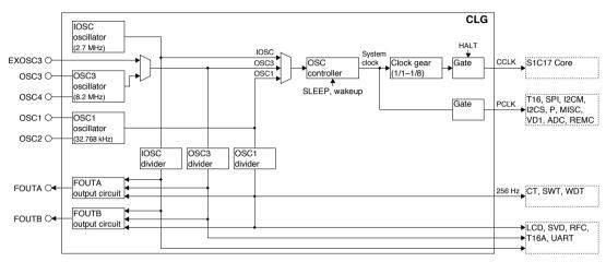
Figure B.1.1 illustrates the S1C17705/703 clock system.
