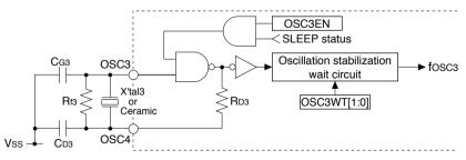
Figure 7.3.2.1 OSC3 Oscillator Circuit
