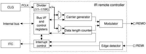
Figure 18.1.1 REMC Module Configuration
