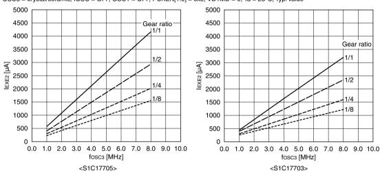
Current consumption-frequency characteristic during execution with OSC3 + clock gear
