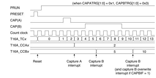
Figure 10.5.4.2 Operation Timing in Capture Mode
