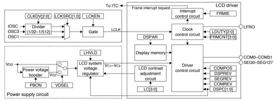
Figure 19.1.1 LCD Driver and Driver Power Supply Configuration
