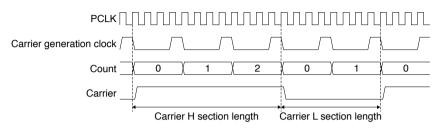
Figure 18.7.1 Carrier Signal Generation
