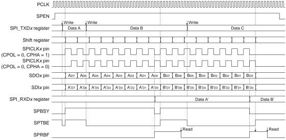
Figure 15.5.2 Data Transferring Timing Chart (MSB first)
