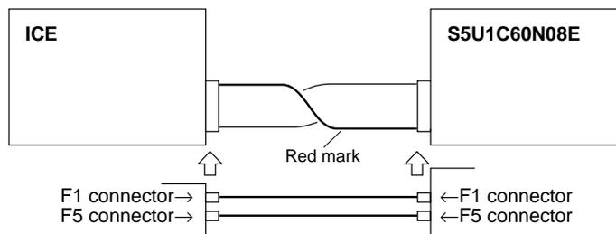
Fig. 4.1.2 Connection diagram
