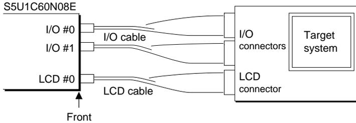
Fig. 4.3.1 Connection of target system
