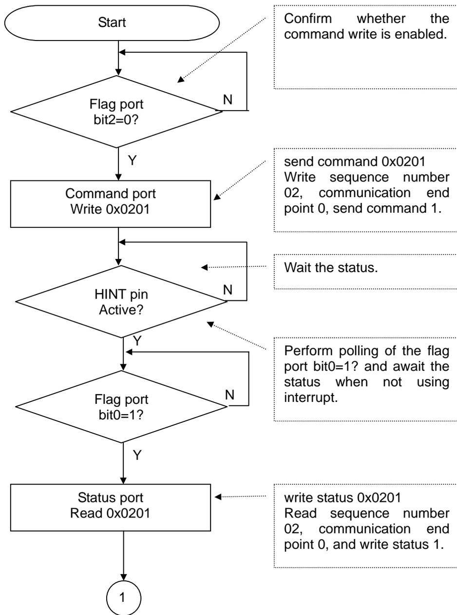
Fig.4.1 MAC address setting flow
