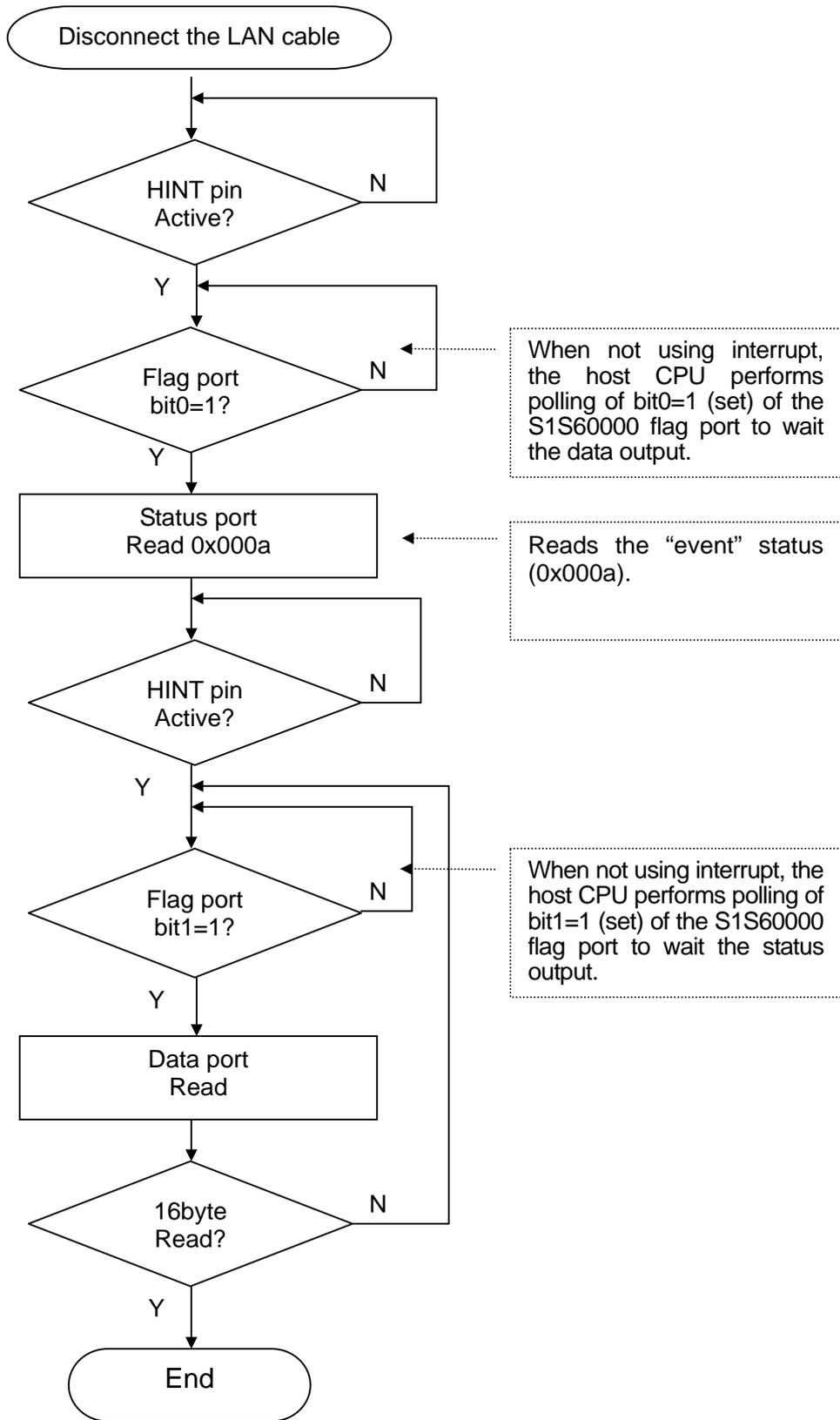
Fig.3.1 Cable disconnection event read flow
