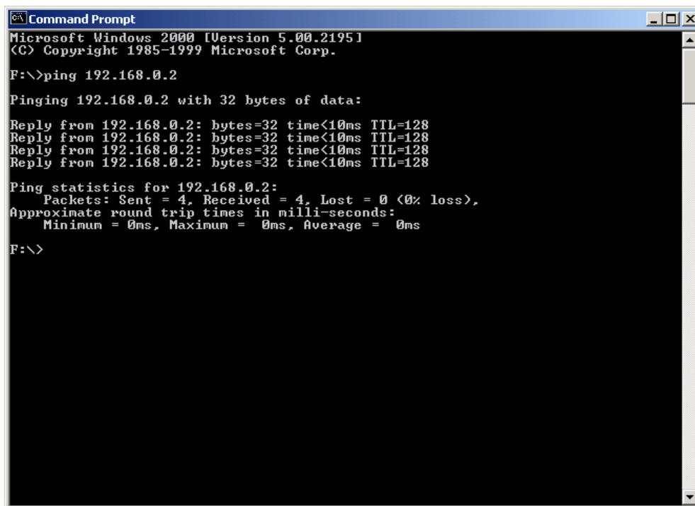
Fig.5.1 Transmission of pings from the PC to S1S60000 and reply to pings
