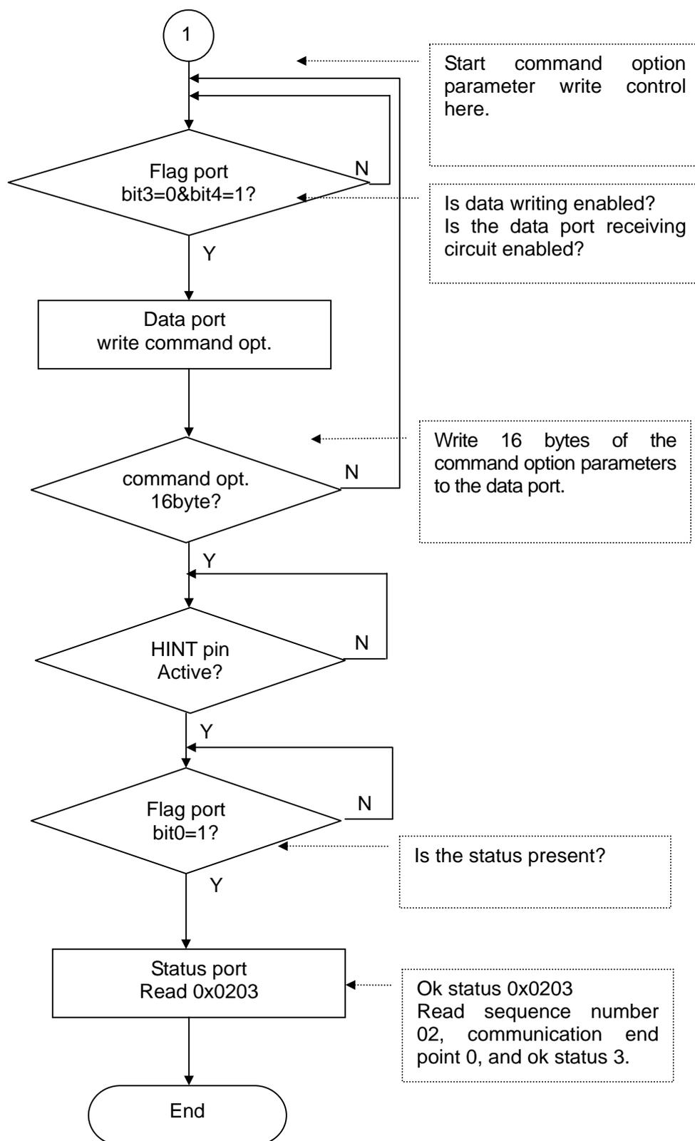
Fig.4.2 MAC address setting flow
