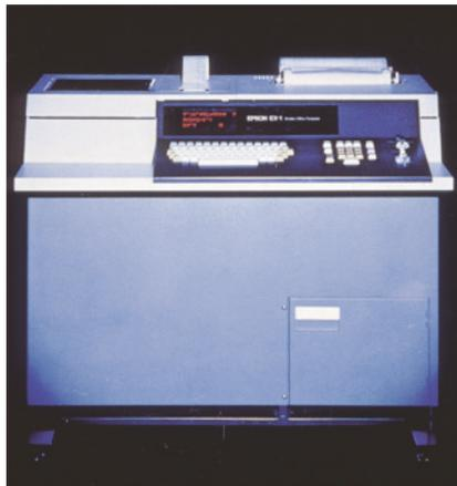
CPU: Intel 8080 8-bit microprocessor
