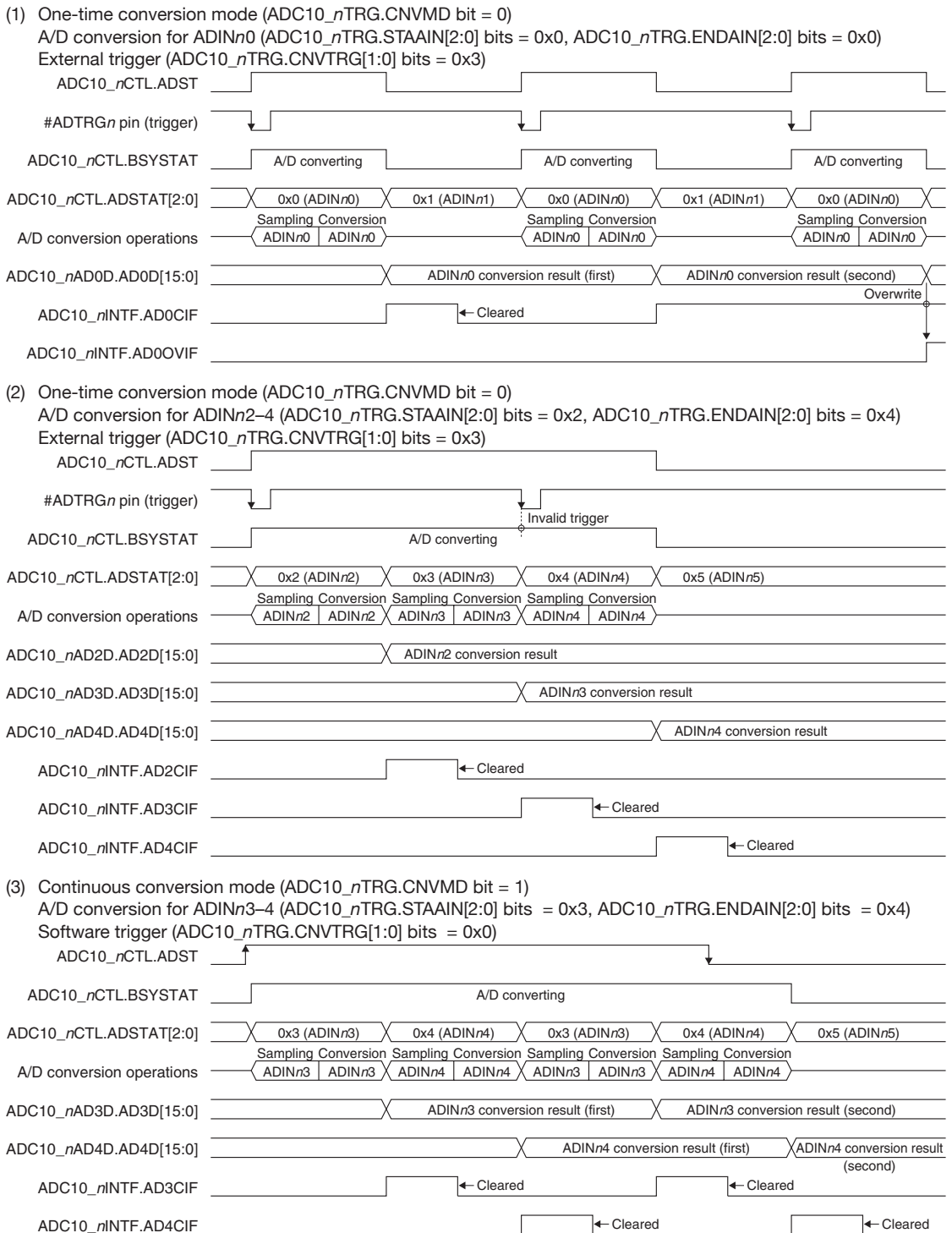
Figure 17.4.4.1 A/D Conversion Operations
