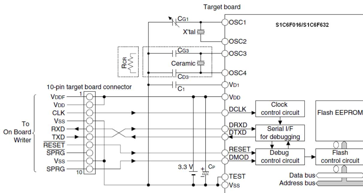
Fig.2.4.1(a) On-board programming connection diagram
