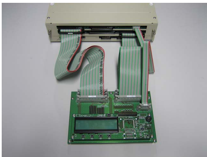
Figure 4.2.1 Connecting the in-circuit emulator
