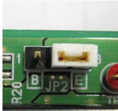
Figure 2.2.1 (b) Switch setting for use of external power supply
