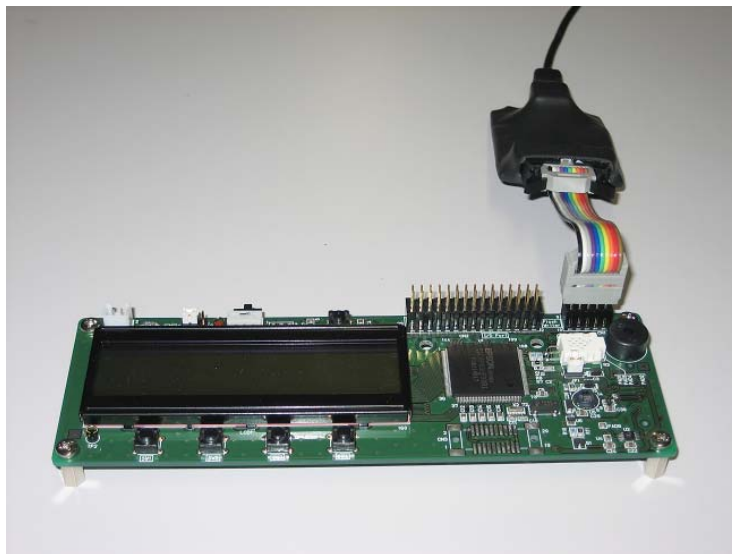
Figure 4.1.1 Connecting the USB-Serial on Board Writer
