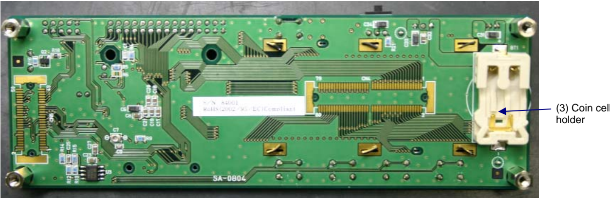
Figure 2.1.2 Names of components mounted on the underside of the S5U1C6F632T1
