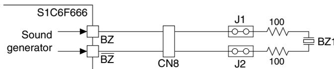
Figure 2.1.5 Buzzer Circuit
