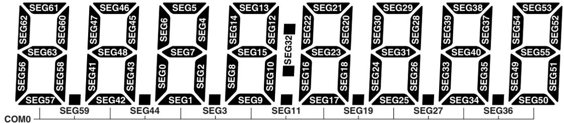
Figure 3.2.2.1 Correspondence between Segment Outputs and LCD Segments
