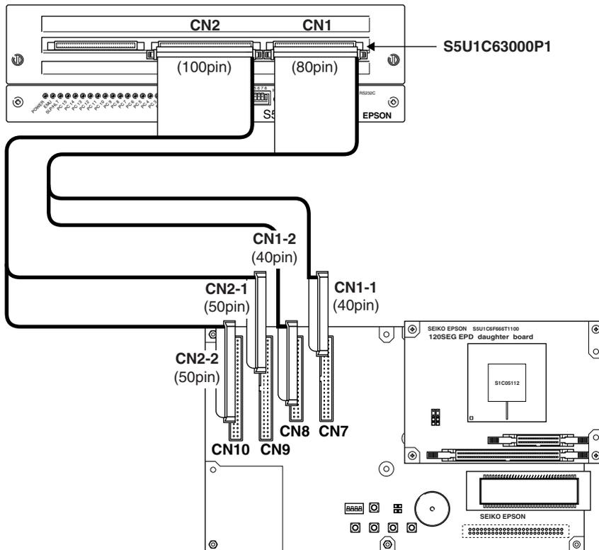
Figure 4.2.1 Connecting to ICE63 (S5U1C63000P1)
