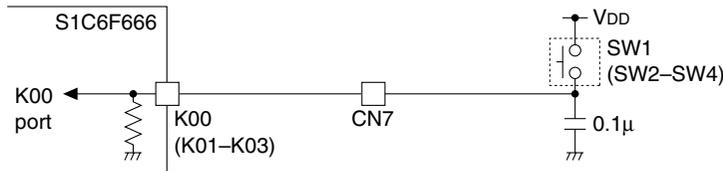
Figure 2.1.2 Switch Input Circuit (SW1–SW4)
