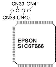
Figure 4.3.1 Motor Driver Output Pads
