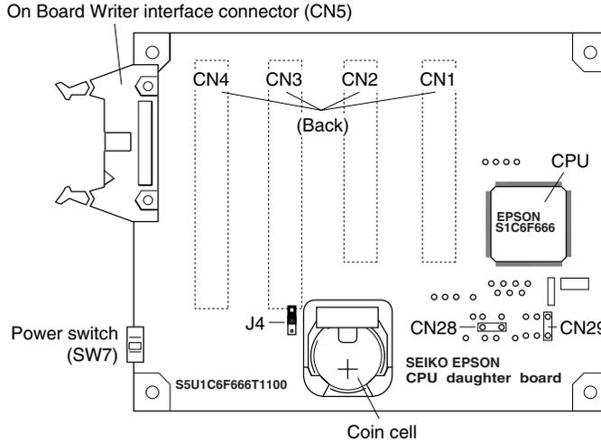
\* The J4 jumper is set to OFF at shipment, change it to ON (short circuit) before using the S5U1C6F666.
