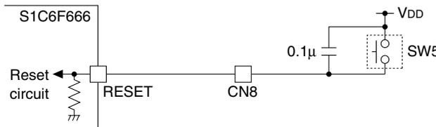
Figure 2.1.3 Reset Input Circuit
