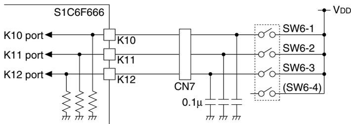
Figure 2.1.4 Switch Input Circuit (SW6)
