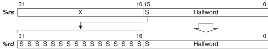
Figure 3.7.1 Signed 16-Bit Transfer (Register → Register)
