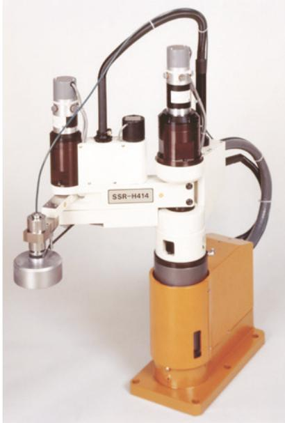
Horizontally articulated (SCARA type) precision assembly robot
